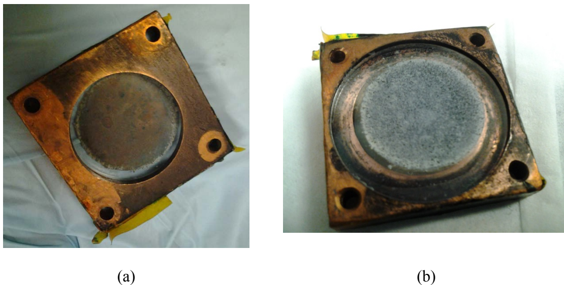
Figure 3.2: (a) Front and (b) back view of one of the windows on the collision cell. The alkali vapor cools down on and coats these components with rubidium and its oxide (white residue) fairly quickly, affecting passage of the probe beam in the process. (See text for more details.)
