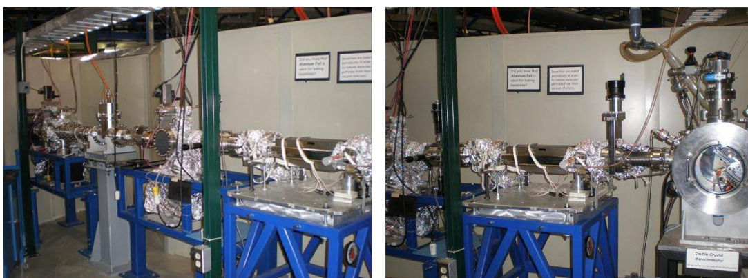
Figure 2.4. DCM (double crystal monochromator) beamline which was used to measure the XANES and EXAFS spectra.
