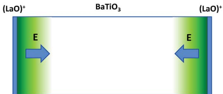
Figure 7.2: Schematic illustration of the charge distribution and the intrinsic electric field in a \text{BaTiO}_3 film terminated with positively charged (\text{LaO})^+ monolayers at the left and right interfaces. A gradient shadow region indicates the screening charge penetrating into \text{BaTiO}_3 . Blue arrows indicate the direction of the intrinsic electric field that has a tendency to pin the local polarization along the field direction.
