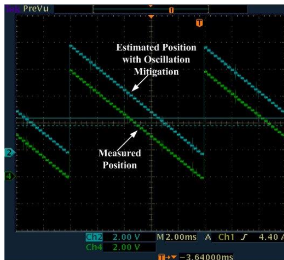
Figure 7.22: Comparison of the measured and estimated rotor positions for \lambda = 0.1 when the rotor speed was 1500 RPM.
