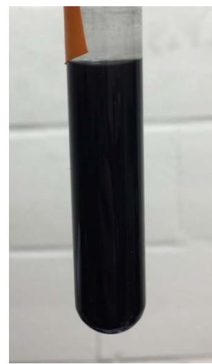
Figure 4.6: Jet-A with 0.1% CNP, 1.5% surfactant. 30 minutes after mixing.
