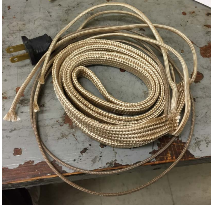
Figure 3.5: 313 Watt heat cable with 120VAC plug.
