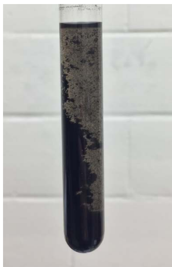
Figure 4.5: Jet-A with 0.1% CNP. No surfactant. 30 minutes after mixing.
