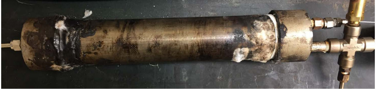
Figure 3.2: Testing chamber without heating apparatus.
