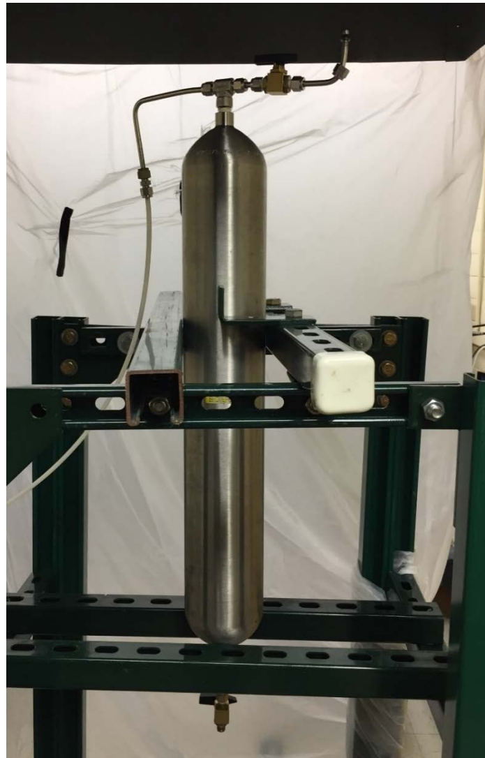
Figure 3.3: Pre-heated fuel vessel.
