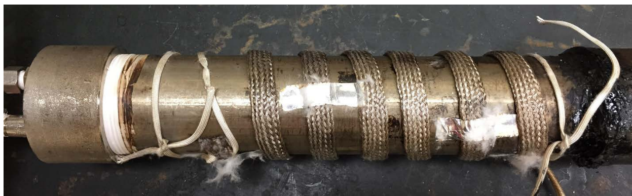
Figure 4.2: Testing chamber with heat cable installed.
