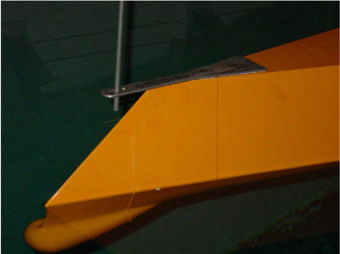
Figure B-1 Rod through slotted hole used a means of supporting the ship in yaw for initial, non-archival round of straight ahead tests. Rod diameter is 0.375 inches.
