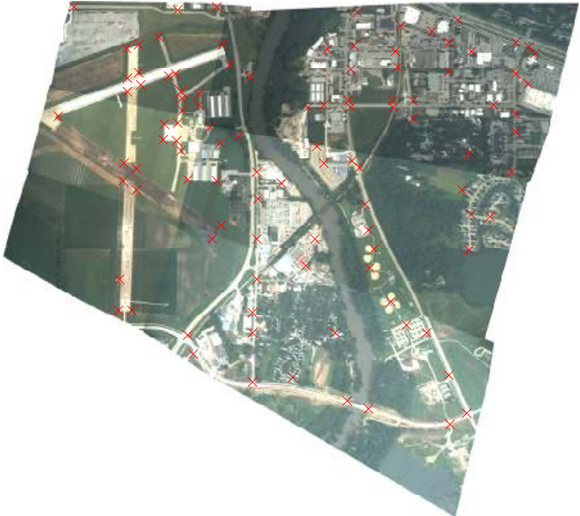
Figure 45: GCPs Used in the Calculation of Image Placement Accuracy. Each GCP is marked with a Red X
