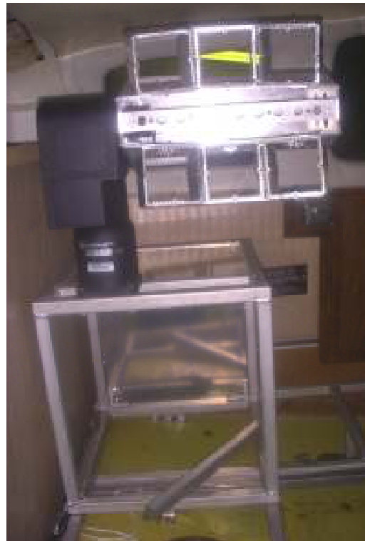
Figure 22: Completed Aft Rack with Camera Pan Tilt Attached
