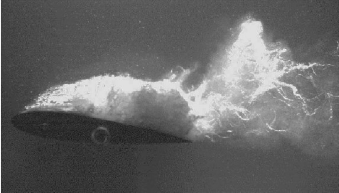
Figure 1: Sheet cavitation on a hydrofoil (Arndt et al. , 2005).
