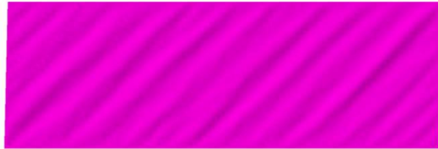
Figure 2.8: Wrinkling under shear force
