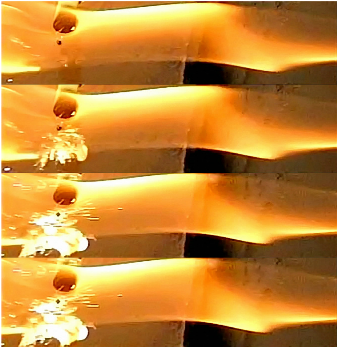
Figure 3-4: Micro-Explosion – High Density Satellite Droplet Concentration Regions Result in Gaseous Cloud like Burning and Low Density Regions Result in Enveloping Flame Burning ( D_o=1.67 mm, MSAR 30% H 2 O, 1200 fps)
