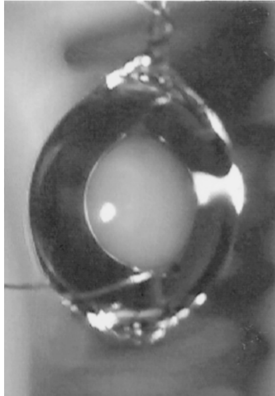
Figure 1-7: The Phase Separation of an n-hexadecane-in-water emulsion droplet
