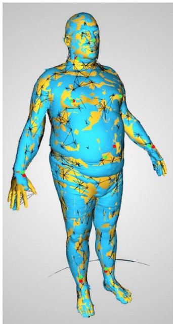
Figure 10: H-Anim markers being used for the registration of a template model to a human body scan
