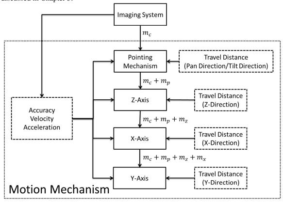
Figure 10: Systems Diagram of the Plant Inspection Robot
