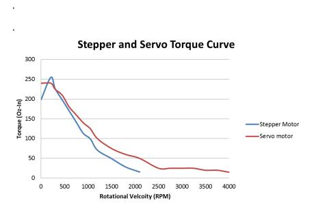
Figure 6: Torque curve of 260 oz-in stepper and 240 oz-in servo
