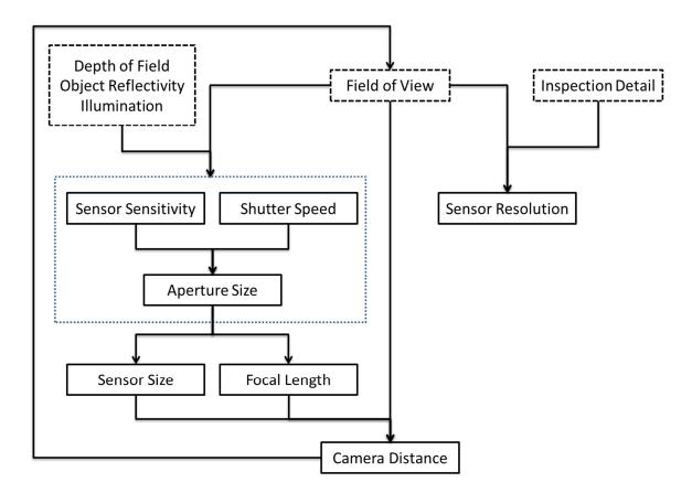
Figure 11: Vision System Design Process
