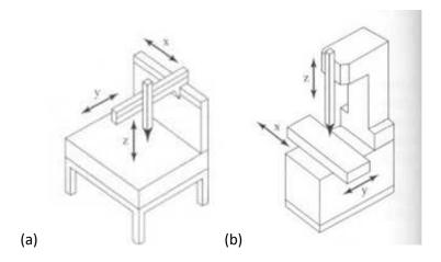
Figure 1: Asymmetrically-supported linear motion structures: cantilever (a) and column (b) (Groover, 2001)
