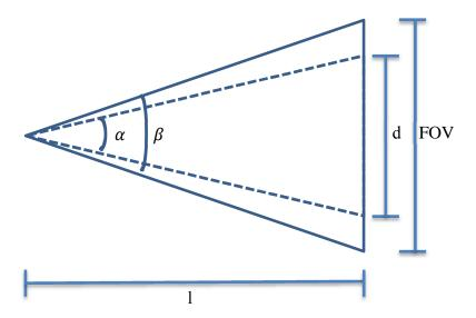
Figure 17: Vertical Angle of View of the Object Height and Vertical Field of View
