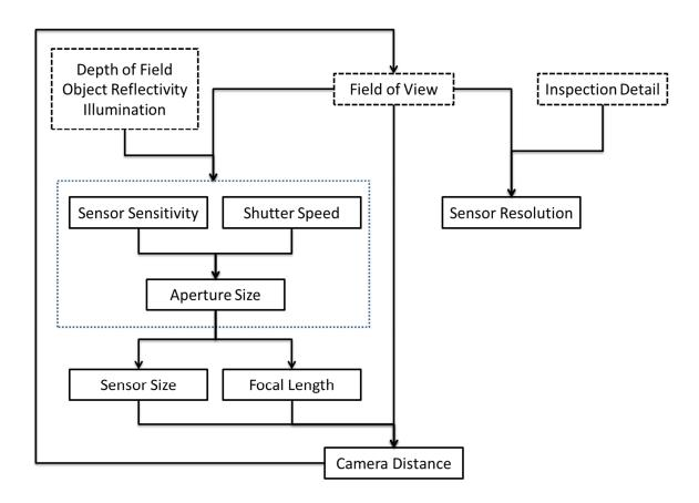
Figure 11: Vision System Design Process
