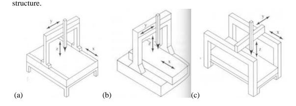
Figure 2: Symmetrically-supported linear motion structures: moving bridge (a), fixed bridge (b) and gantry (c) (Groover, 2001)
