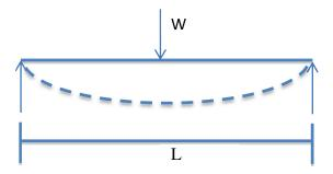
Figure 19: Diagram of a simply supported beam with length (L) with load (W)
