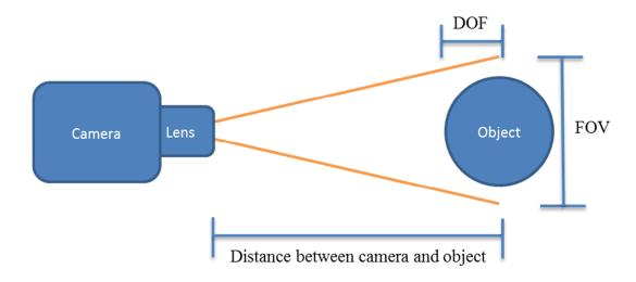
Figure 12: General parameters of a vision system
