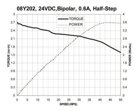
Figure 27: Anaheim Automation 08Y202 Torque Curve
