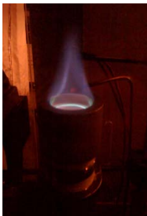
Figure 2-7: Fuel Burn Off at the Reactor Exit.
