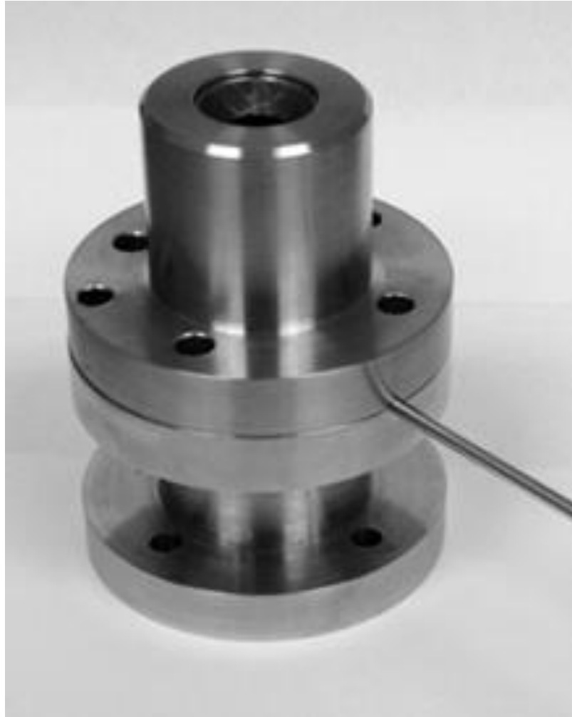
Figure 3.3 Detail of fuel nozzle and air swirler assembly
