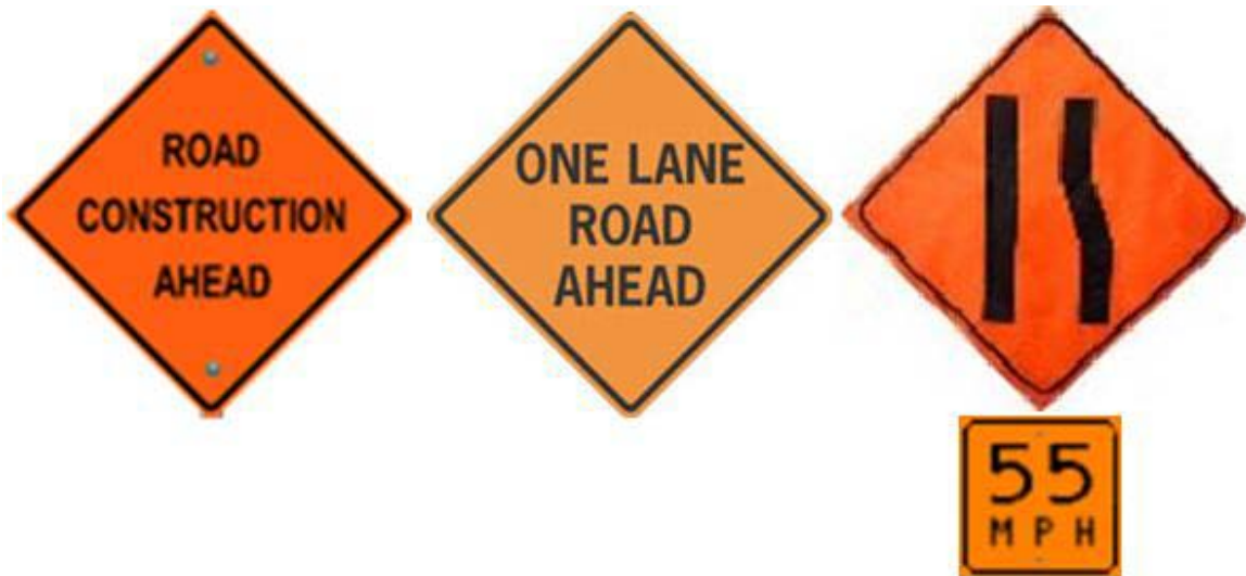
Figure 3. Signs in the advance warning area of the work zone
