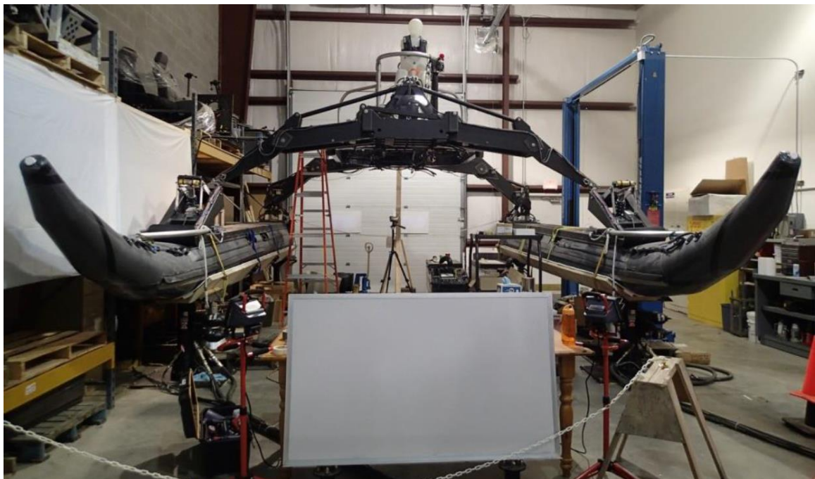
Figure 2-10 2-post shaker rig experimental setup [16]
