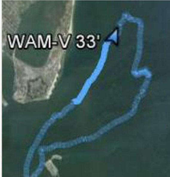
Figure 2-16 Sea-trial trajectory for WAM-V rough -water testing and the direction of dominant waves
