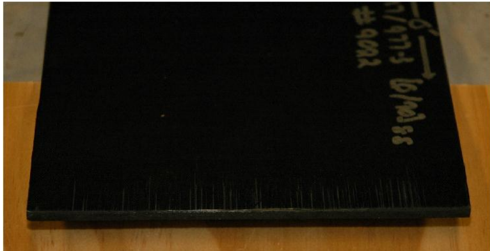
Figure 2.5: Image of a sample cut using table saw
