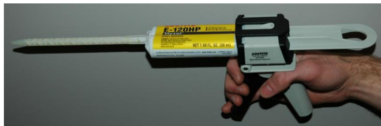
Figure 3.8: Epoxy application system (McAndrew, 2009)
