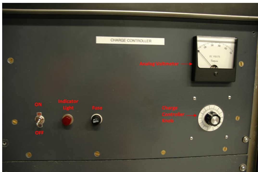
Figure 5.5: Left panel of the current pulse generator (Hart, 2011)
