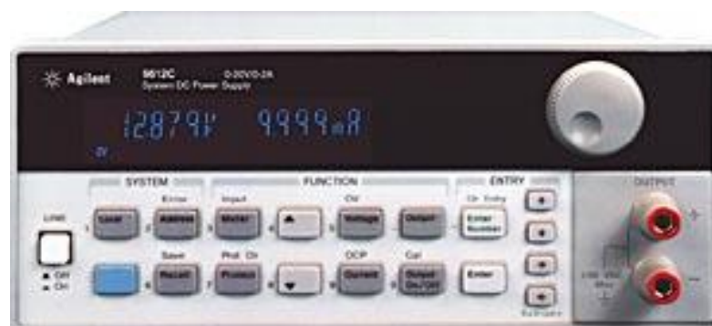
Figure 3.4: HP 6612C DC Power Supply (Axiom, 2011)
