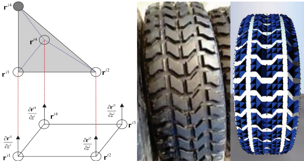
Figure 4.3: (Left) The formation of solid tread blocks by using the same nodes to describe the shear deformable shell elements and the co-rotational elements connectivity. (Middle) The tread pattern of a sample off-road tire, the Goodyear Wrangler MT. (Right) The emulation of the of the sample off-road tire tread pattern created from co-rotational tetrahedral elements on the shear deformable shell element tire model
