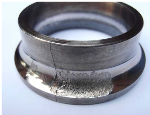
Fig. 1.2: Axial cracking on bearing ring.
