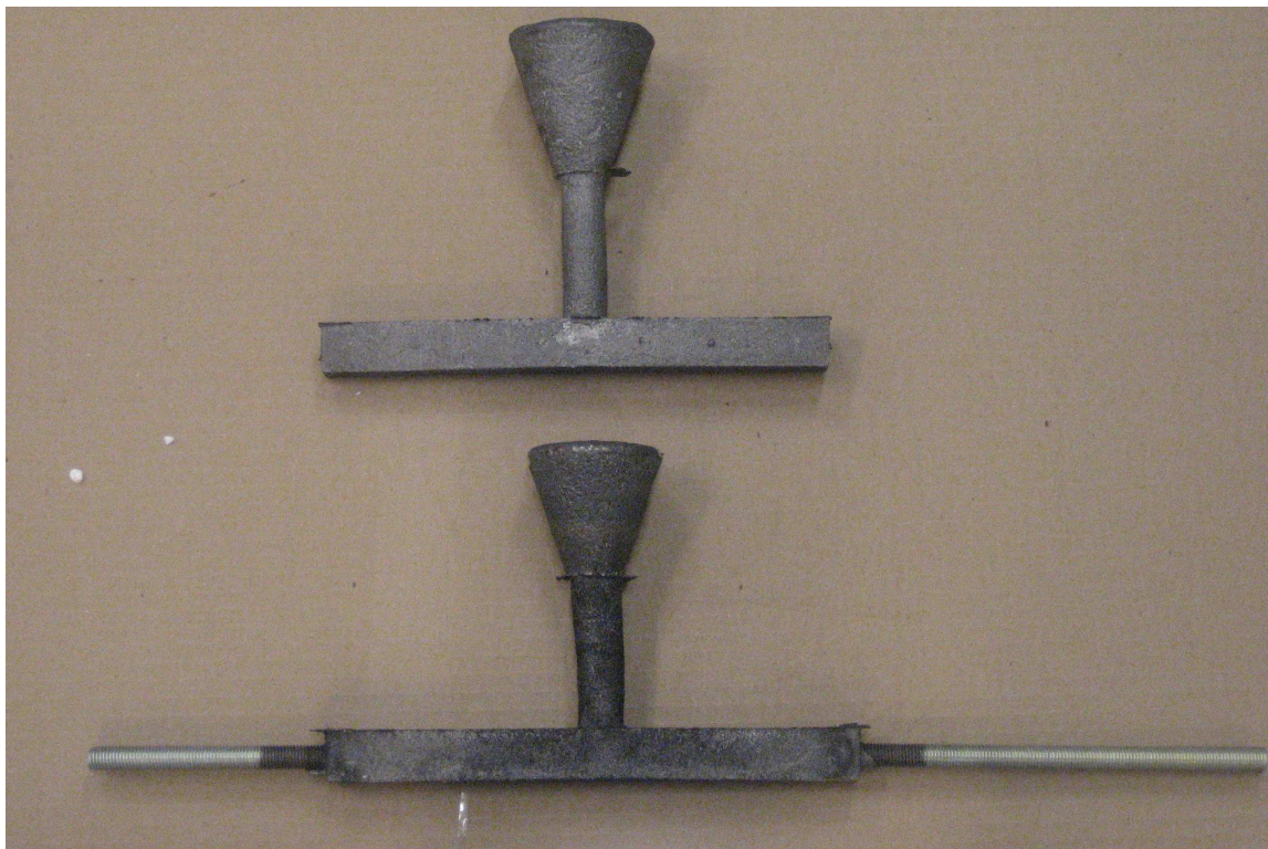
Figure 3.4. Examples of the Unrestrained and Strained castings.
