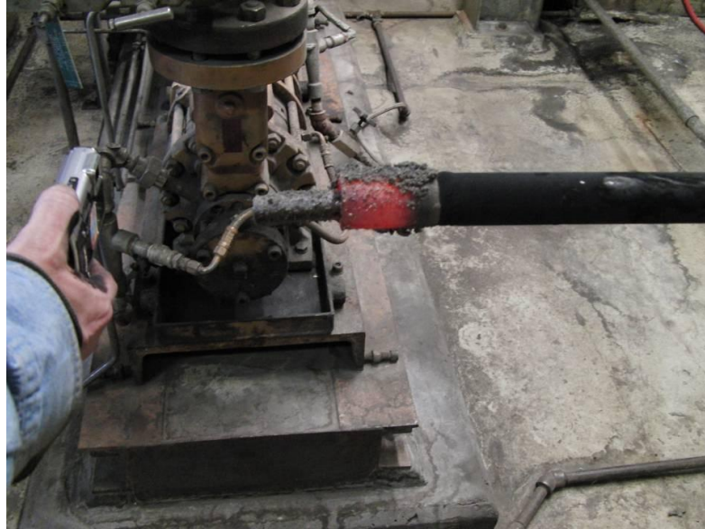
Figure 4.8 The front end of the probe is pulled out from the window
