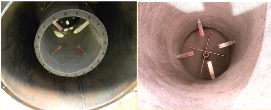
Figure 2.5 : Inner view of the gasifier (bottom view-left and top view-right)
