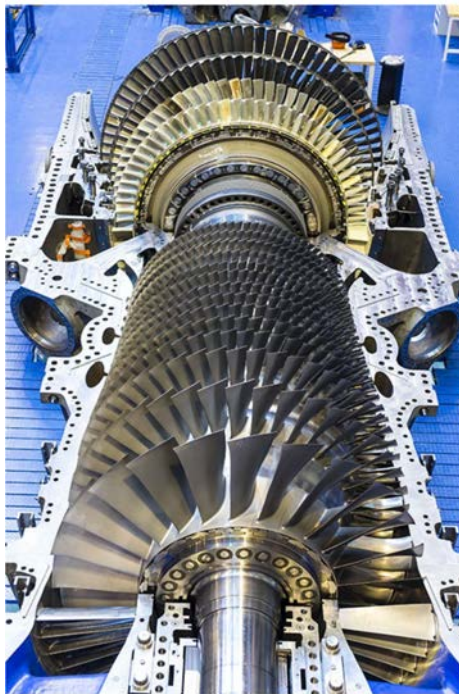
Figure 1.10 : Ge's class E syngas turbine [26]
