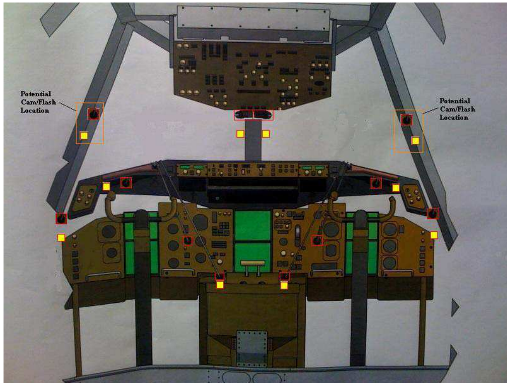
Figure 20. IFD SE Camera and Illuminator Locations
