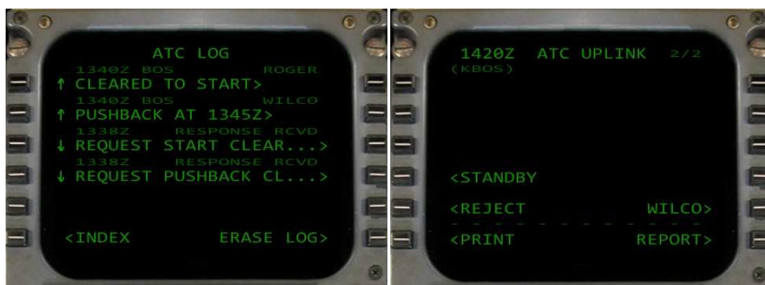
Figure 14. ATC Log (left) and Downlink Response (right) pages
