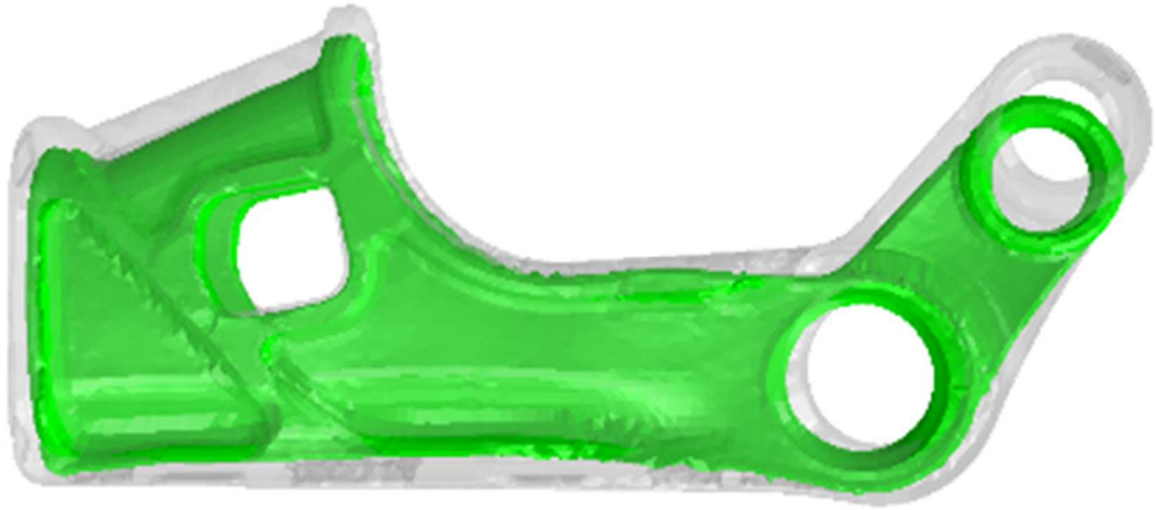
Figure 6.4 Deformed casting at room temperature.
