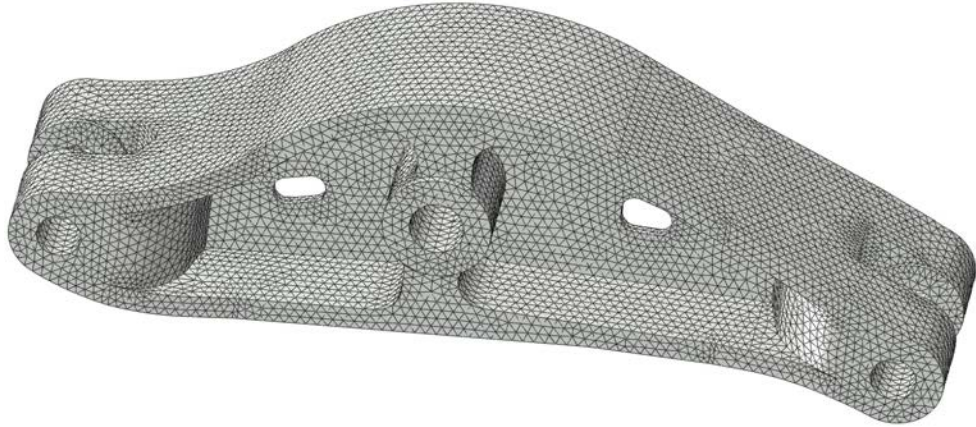
Figure 4.7: An FEA mesh of a lever arm
