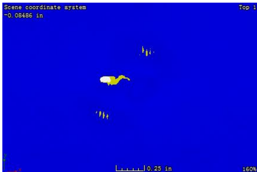
Figure B. 38: CT image at the plane located 3.57 mm away from the impacted surface of sample 1-5
