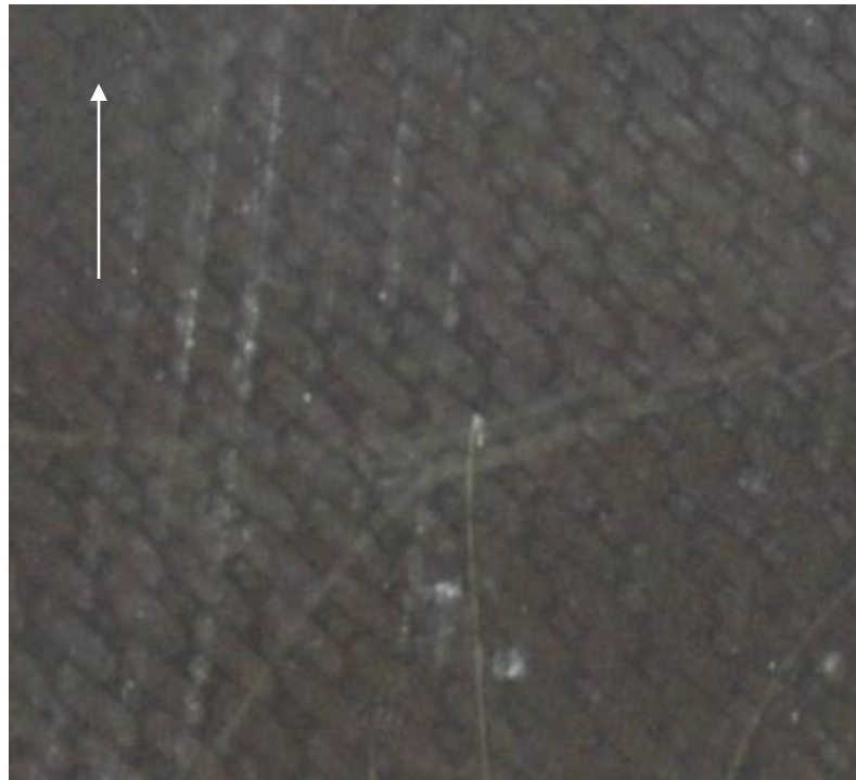
Figure 2. 7: Textile of the Specimen (the arrow indicates a 0^\circ direction)
