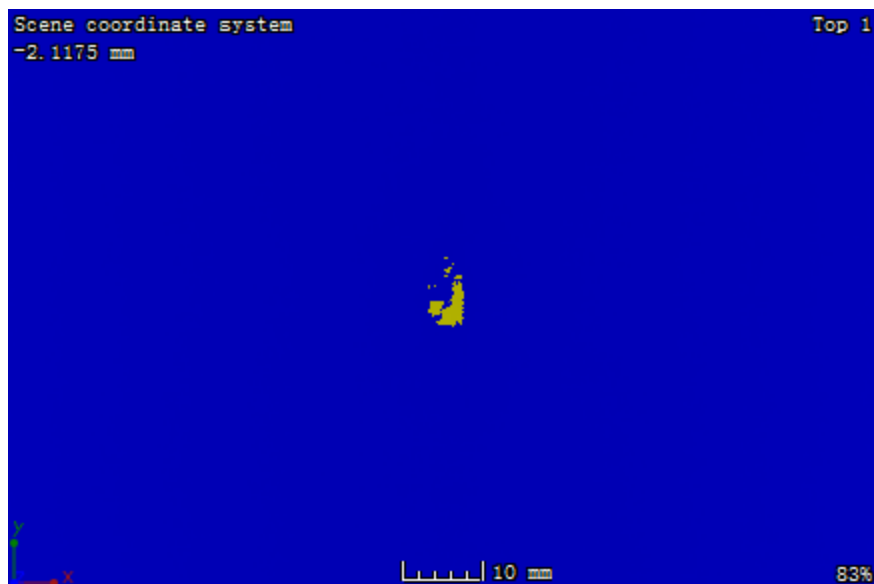
Figure A. 20: CT image at the plane located 2.37 mm away from the impacted surface of sample 2-3
