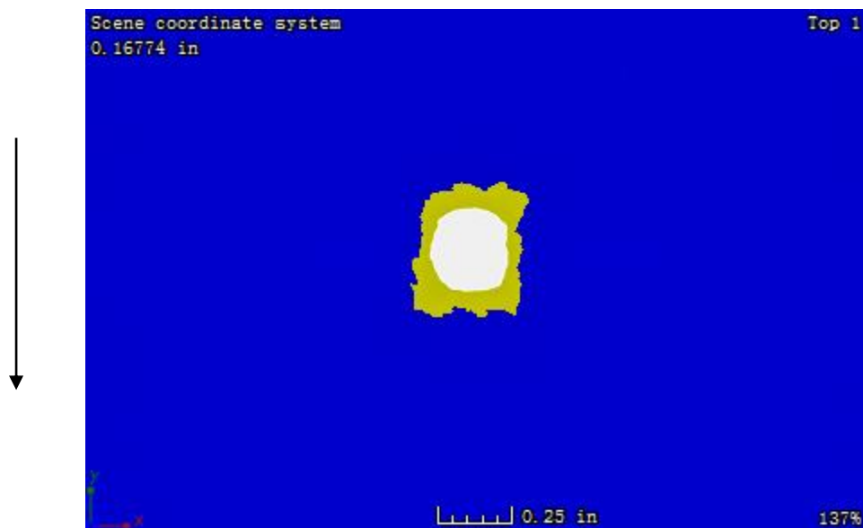
Figure B. 42: CT image at the plane located 0.22 mm away from the impacted surface of sample 1-6
