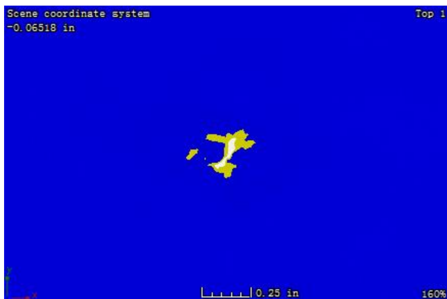
Figure B. 36: CT image at the plane located 3.12 mm away from the impacted surface of sample 1-5
