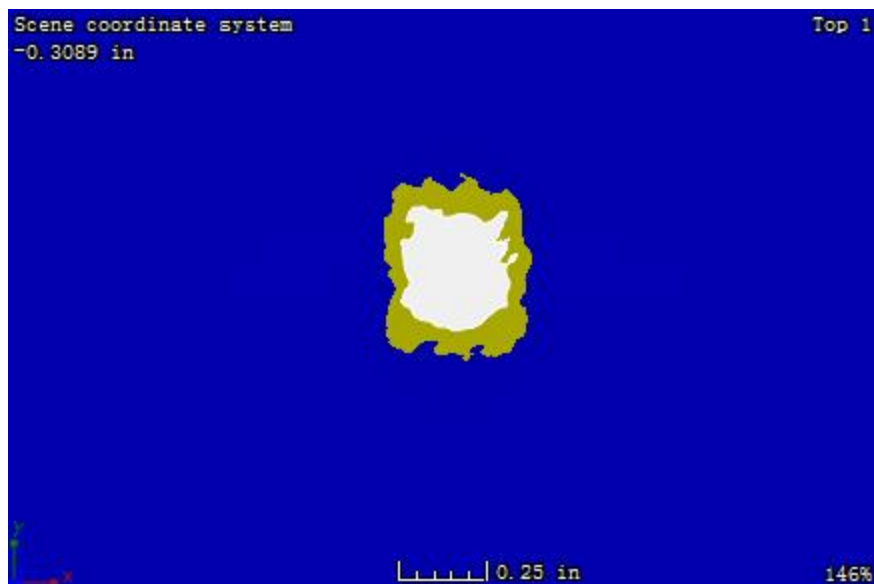
Figure C. 21: CT image at the plane located 0.47 mm away from the impacted surface of sample 2-5
