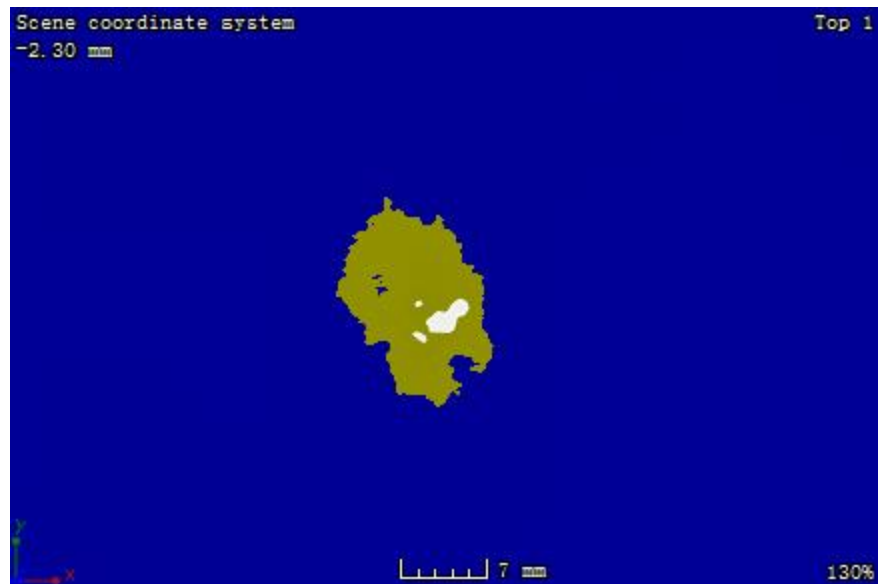
Figure B. 5: CT image at the plane located 0.47 mm away from the impacted surface of sample 1-4
