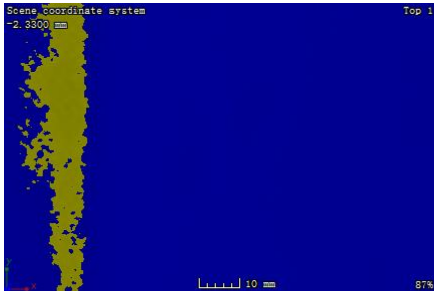
Figure A. 13: CT image at the plane located 3.87 mm away from the impacted surface of sample 2-2
