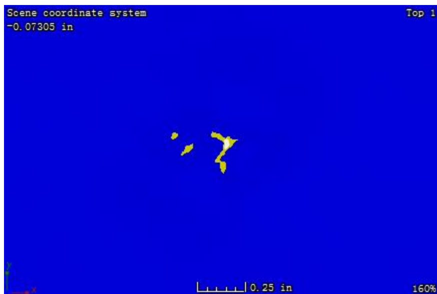
Figure B. 38: CT image at the plane located 3.57 mm away from the impacted surface of sample 1-5
