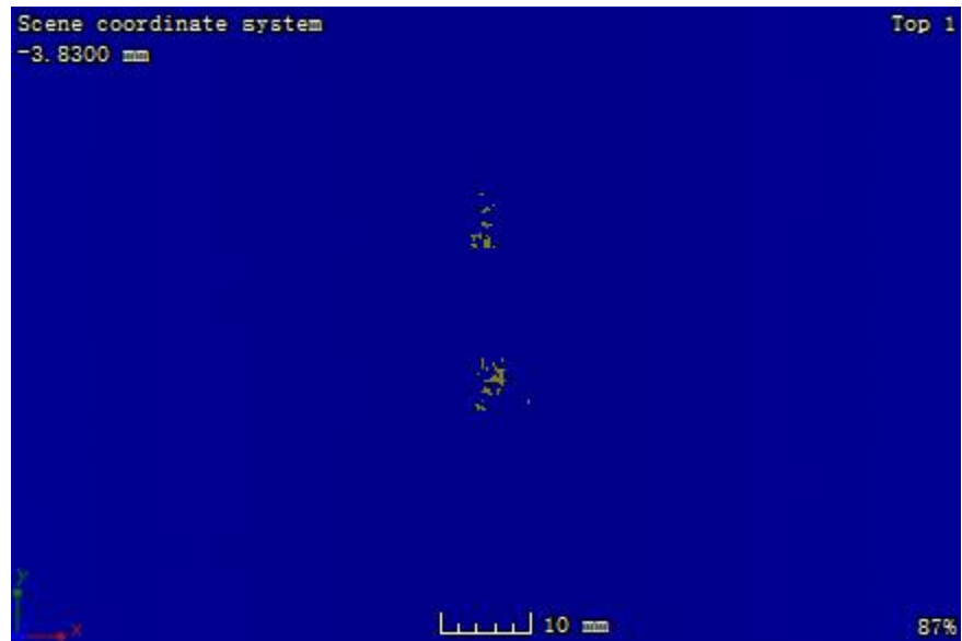
Figure A. 11: CT image at the plane located 2.37 mm away from the impacted surface of sample 2-2
