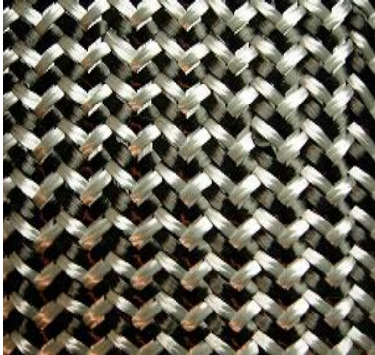
Figure 1. 7: Braided carbon fabrics (A&P Technology, 2013)
