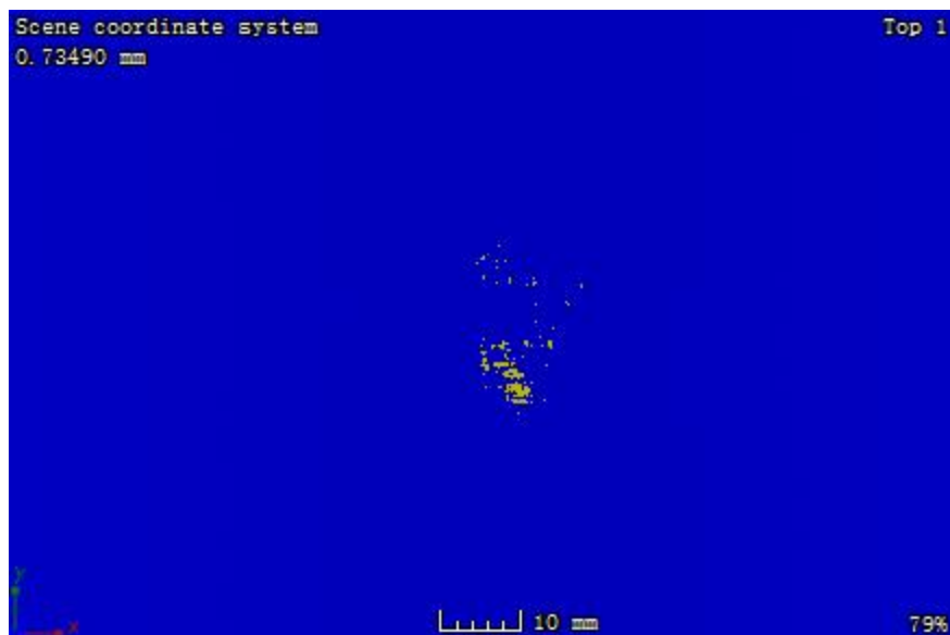
Figure A. 2: CT image at the plane located 0.22 mm away from the impacted surface of sample 2-1
