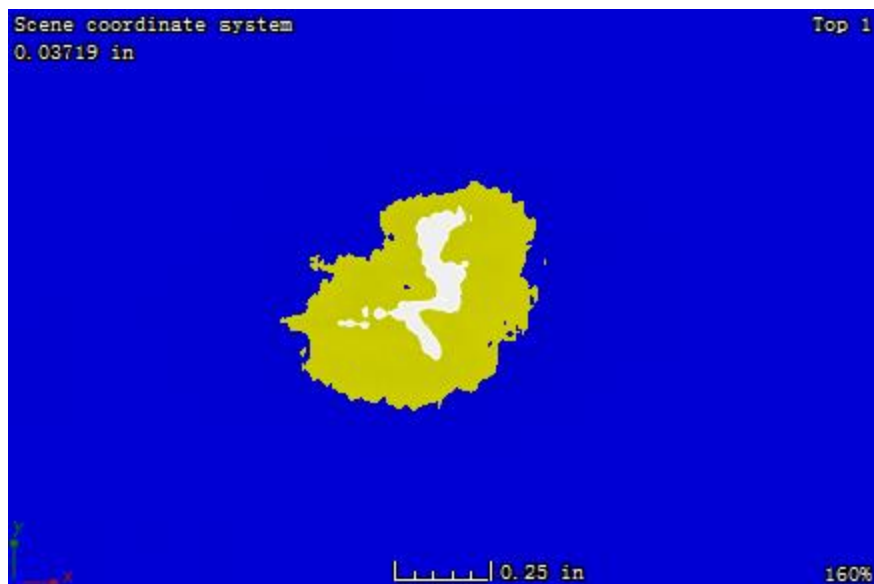
Figure B. 26: CT image at the plane located 0.62 mm away from the impacted surface of sample 1-5
