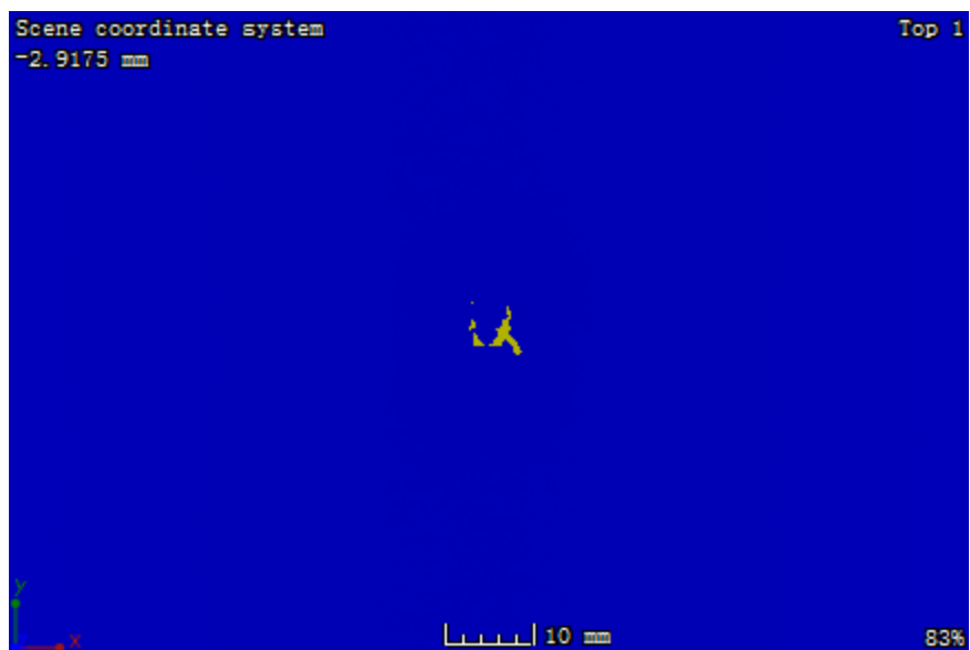
Figure A. 18: CT image at the plane located 1.87 mm away from the impacted surface of sample 2-3
