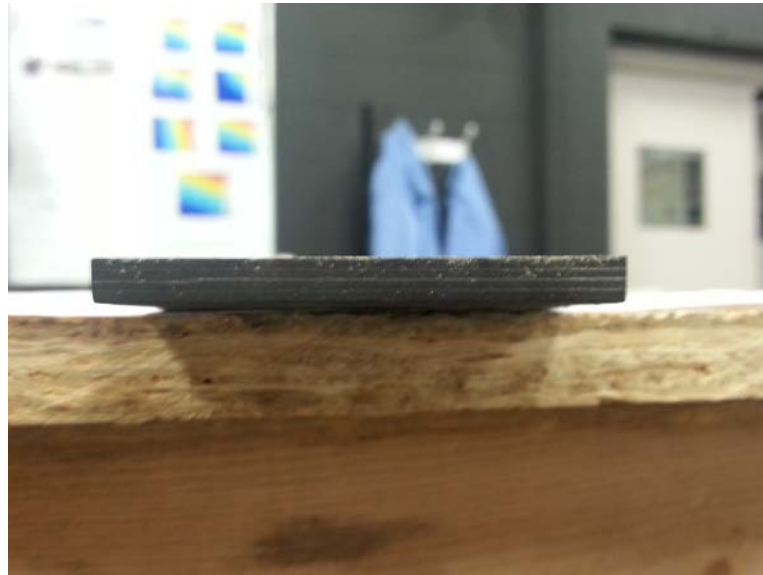
Figure 4.38: Delamination Side 3 of Sample 1-7
