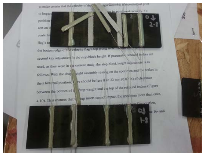
Figure 4.26: Broken Electrodes on Samples 1-8 and 2-8
