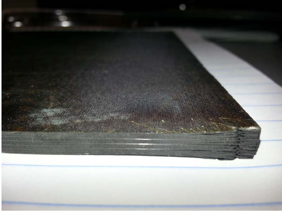
Figure 2.4: Delamination in One of the Samples
