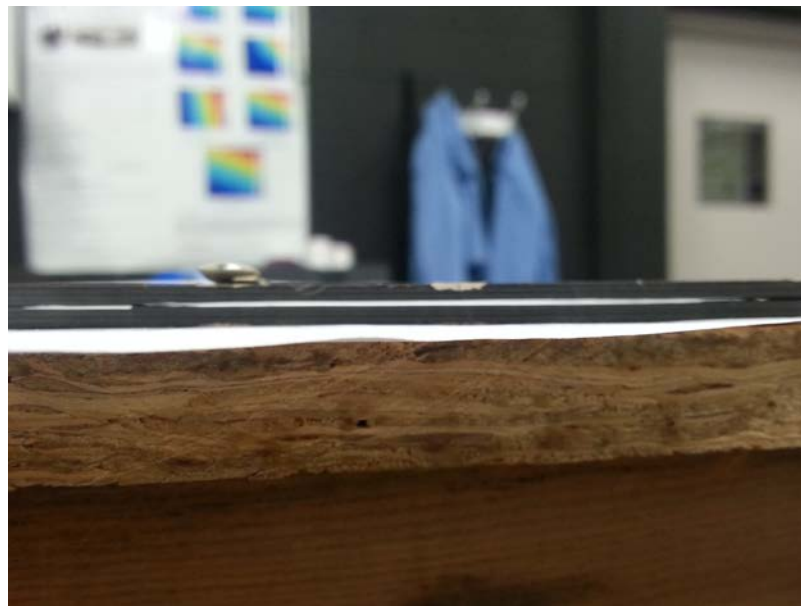
Figure 4.37: Delamination Side 2 of Sample 1-7
