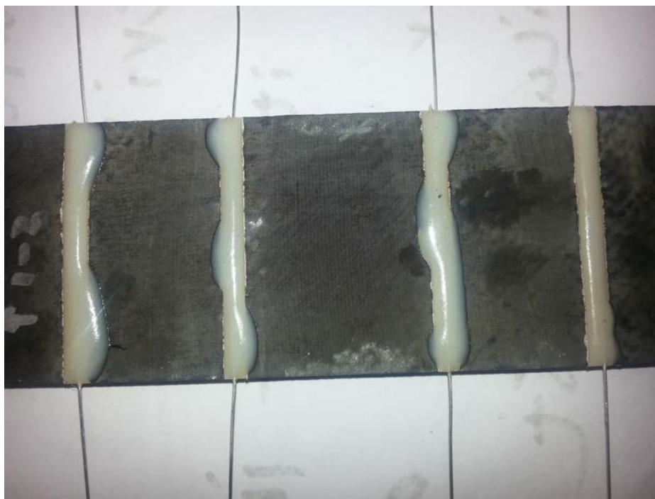
Figure 4.24: Sample 1-8 Bottom Surface after 2 nd Impact
