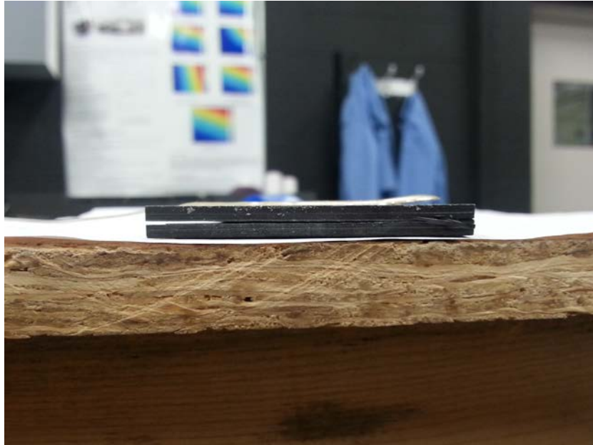
Figure 4.36: Side 1 Delamination of Sample 1-7
