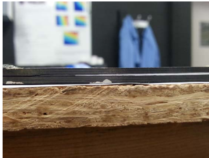
Figure 4.39: Delamination Side 4 of Sample 1-7
