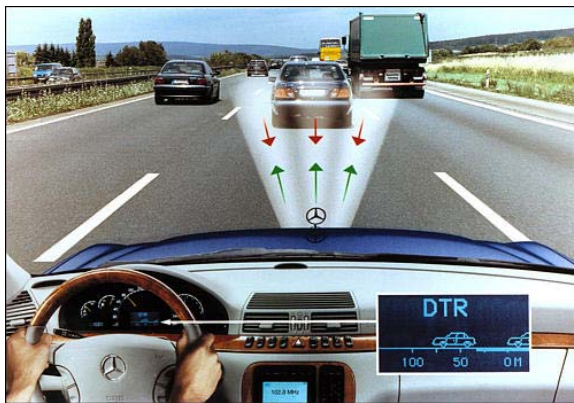
Figure 8. Schematics of the Richardson et al. (2000) and King et al. (2000) ACC interfaces, respectively. Note: for the Richardson et al. (2000) interface, no visual is provided so the photograph shown is assumed consistent to the interface description provided in the text.
