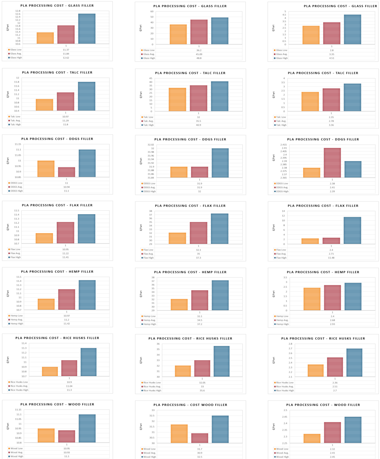
Figure 2.12. Overall processing cost sensitivity analysis. Column 1 is relative to 0.01 kg part weight; column 2 is relative to 0.1 kg part weight; column 3 is relative to 1 kg part weight
