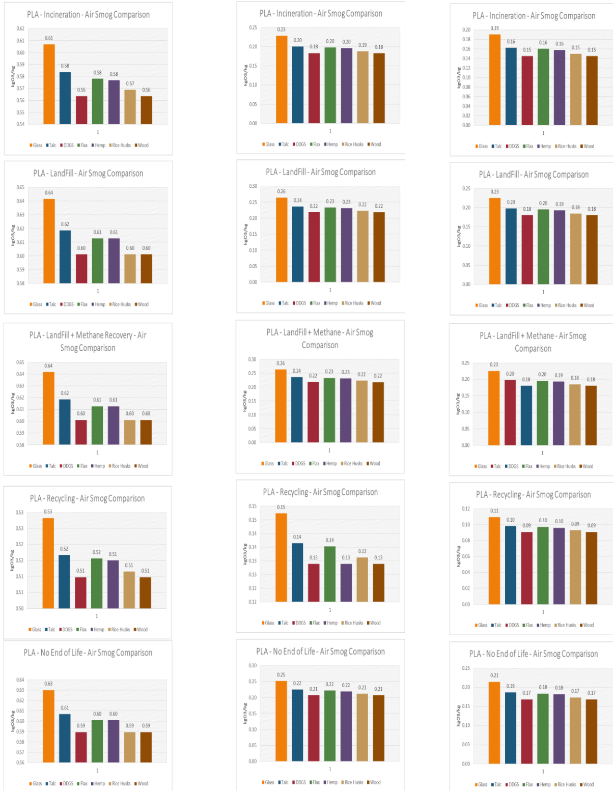
Figure 2.9. Air Smog [kg O 3 /kg] comparison matrix plots, end of life treatments (I, L, LM, R, N) are compared vertically, while part weight (0.01 kg, 0.1 kg, and 1 kg) is compared horizontally
