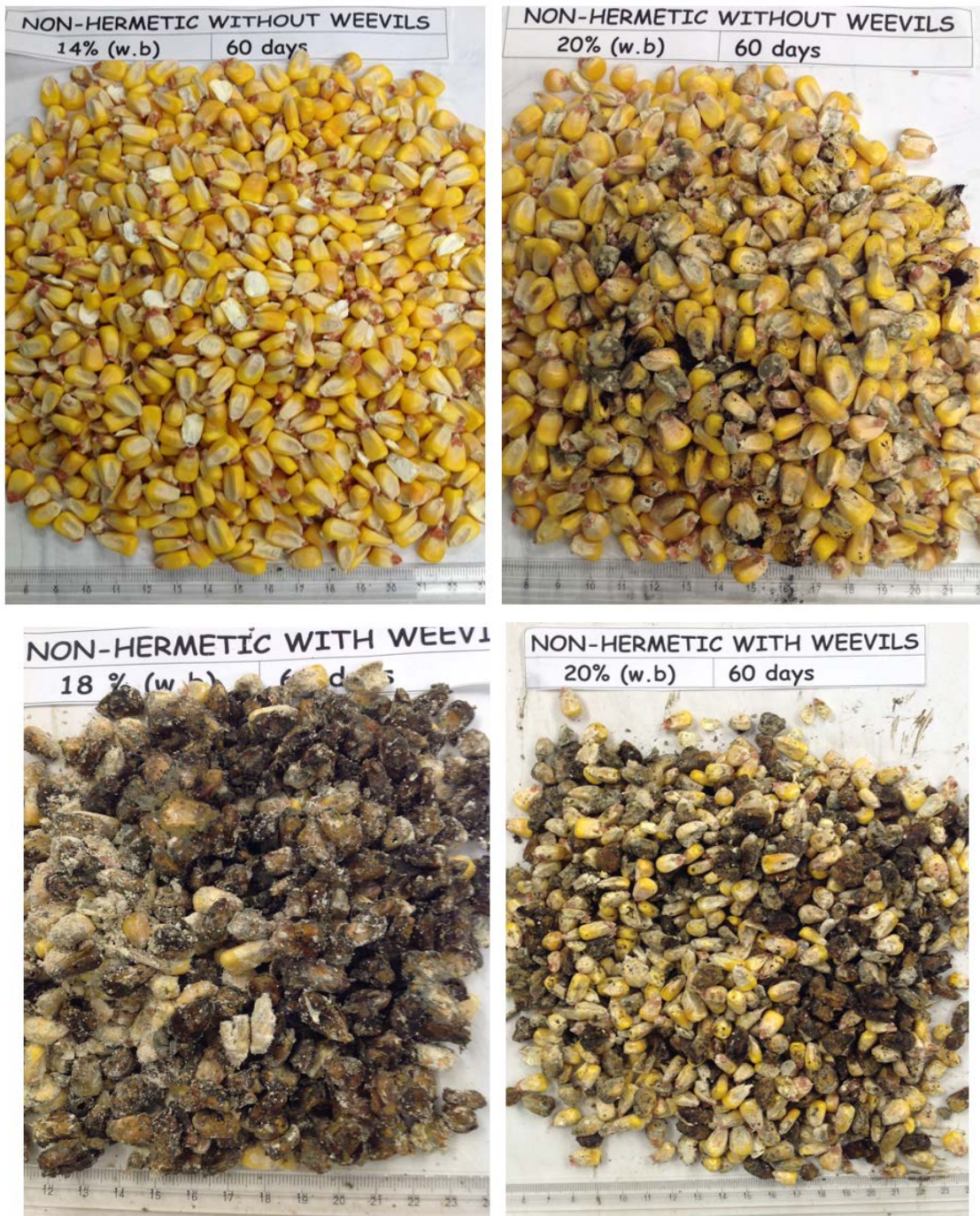
Figure 70. Visible mold growth under non-hermetic without weevils at different M.C % at 60 days of storage.
