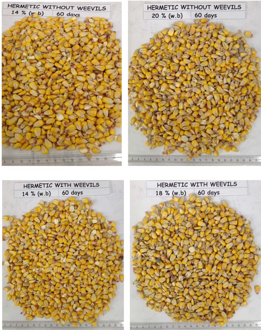
Figure 69. Visible Mold Growth under Hermetic Without Weevils at Different M.C % at 60 Days of Storage.
