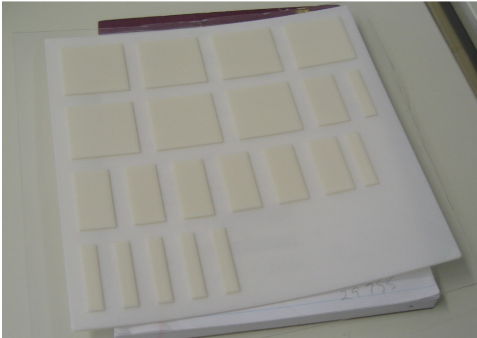
Figure 1 FDM Blanks at 10, 25, and 50mm
