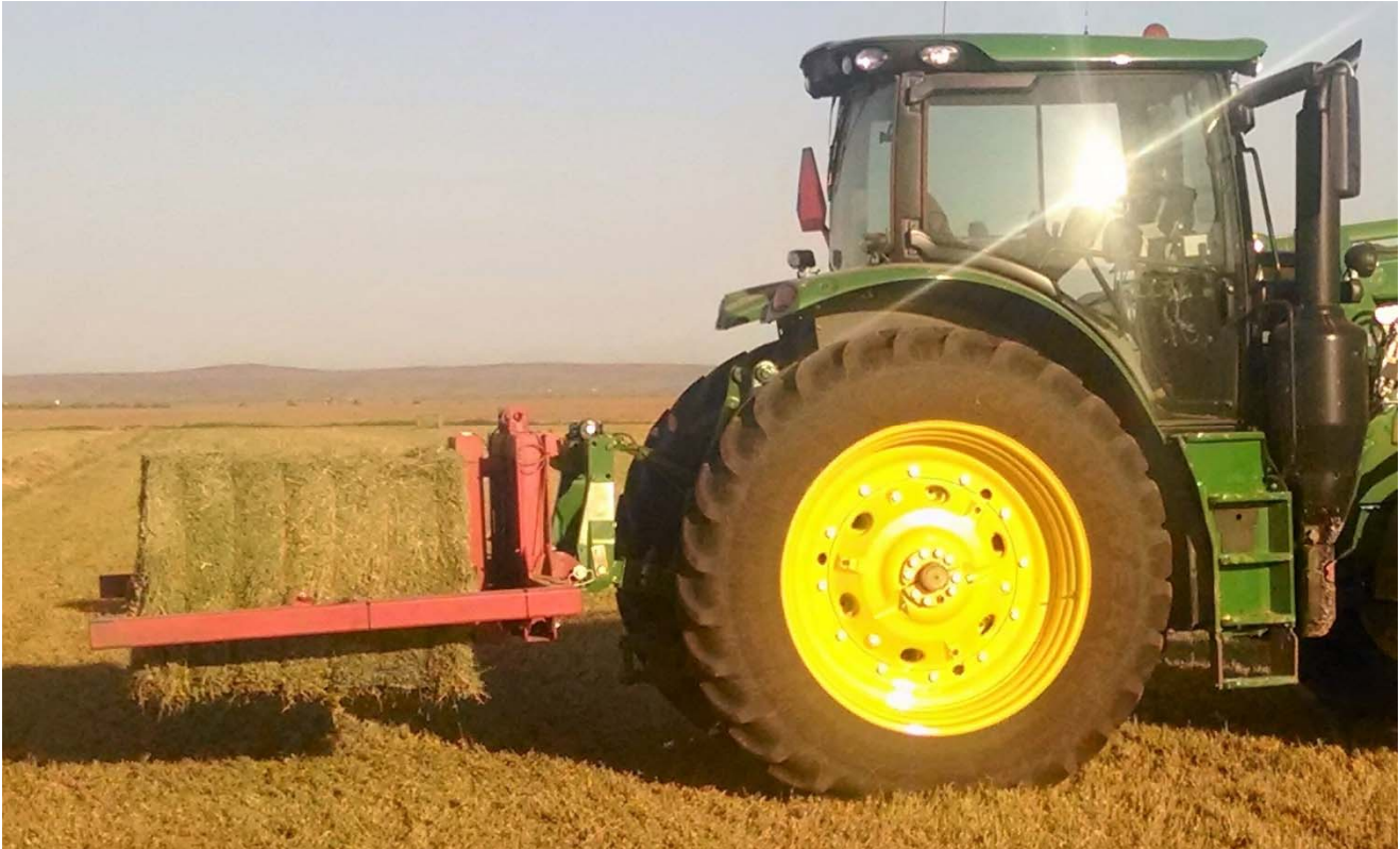
Figure 4.3: A three-point scale attachment used to obtain bale weights. Forks attached to load cells were used to lift the bale off the ground and obtain a weight.
