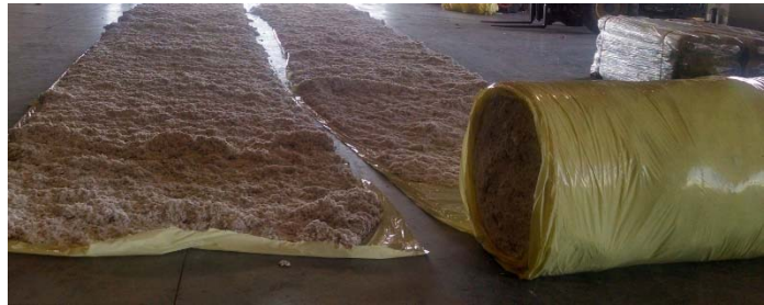
Figure 3.3: A lab test in which plastic wrap was rolled in with each layer of cotton into a module such that the layers could be visualized and unfolded. In the compressed state within the module the layers ranged from 0.64 to 3.8 cm [0.25 to 1.5 in] thick.
