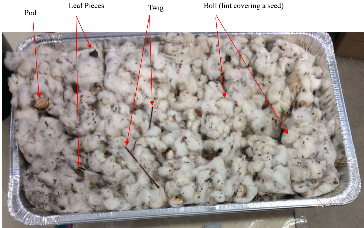
Figure 2.1: Typical sample of cotton from a round bale cotton stripper harvester with diverse mixture of constituents. The relative composition of samples used in this work was seen to change across machine types (picker/stripper), crop varieties, and geographic regions. The clumpy texture of the materials is due to the nature of how the bolls form with lint surrounding the seed.
