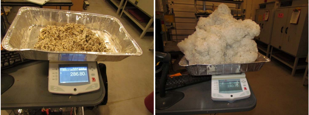
Figure 2.5: 287g of seed (left) and 241g of lint (right) after ginning a sample. The large disparity in bulk density between these two constituents makes cotton turnout a variable of great interest when examining and quantifying the dielectric properties of raw cotton.
