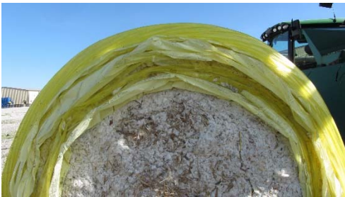
Figure 3.3: A lab test in which plastic wrap was rolled in with each layer of cotton into a module such that the layers could be visualized and unfolded. In the compressed state within the module the layers ranged from 0.64 to 3.8 cm [0.25 to 1.5 in] thick.
