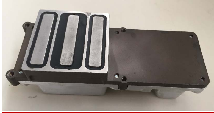
Figure 3.1: Mobil sensor includes probe packaged with electronics and can be mounted on-machine.
