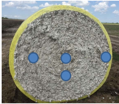
Figure 3.5: Example of sampling points from a round module per protocol. At least four different layers, corresponding to different radii, were sampled at quadrants around the module.
