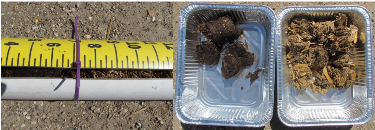
Figure 4.8: Side moisture penetration measurement and separated sample
