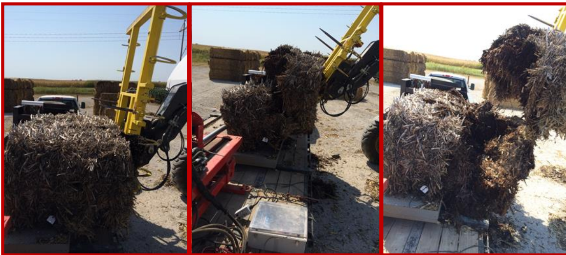
Figure 4.24: Telehandler attempting to pick up a top bale post storage, highlighting loss of integrity
