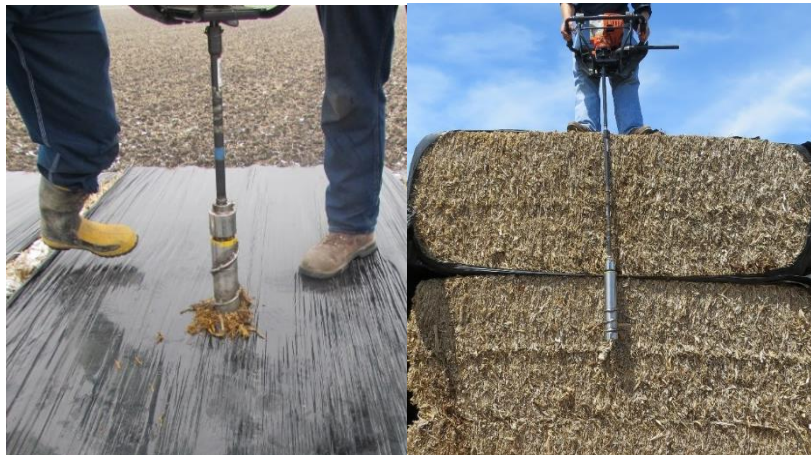
Figure 4.5: Auger coring unit capable of coring 1.2m (4ft) in depth
