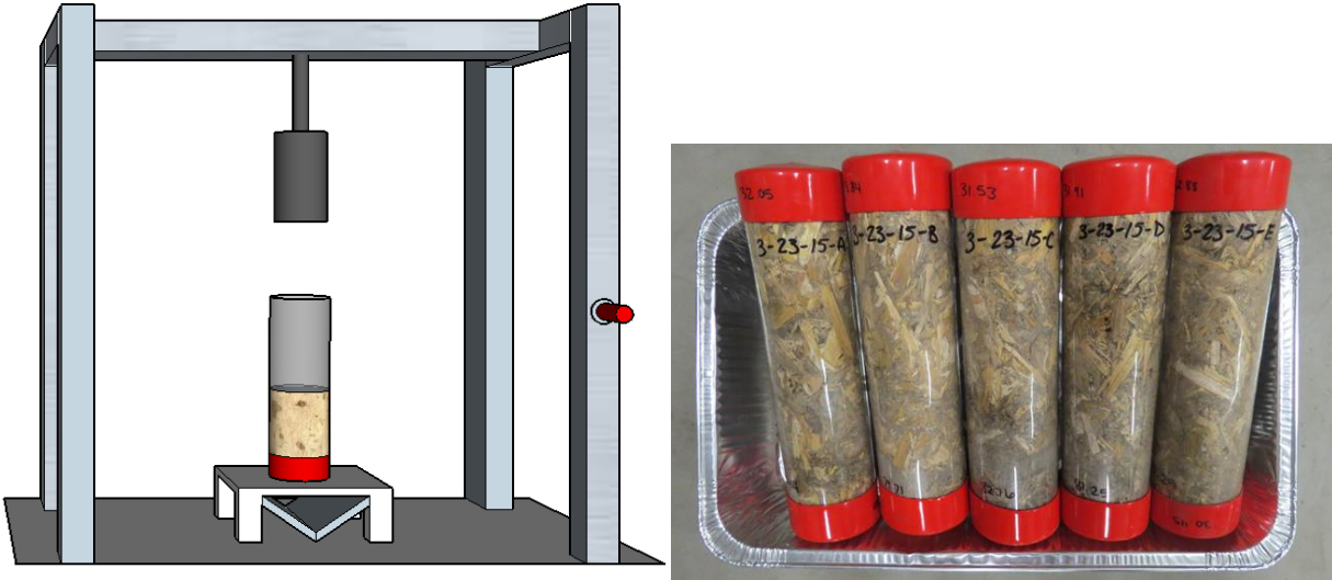
Figure 3.1: Hydraulic press and resultant tubes of densified corn stover.
