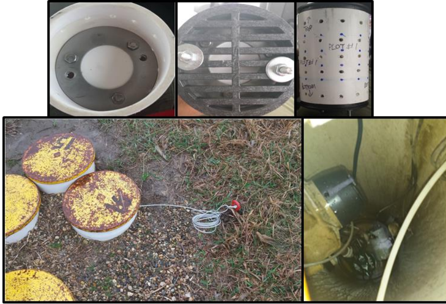
Figure 5.2 Fabricated POCIS canister, and installation of POCIS at Nashua tile sump.
