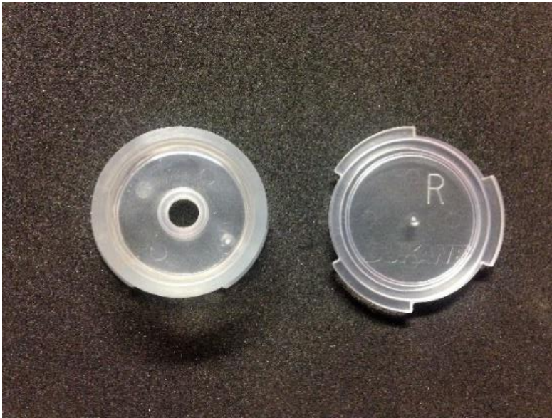
Figure 3.9. PLA Rigid Sample (Ingeo 2003D).
