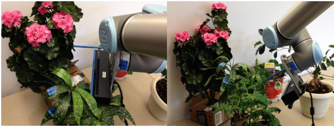
Figure 10. Probing examples. Left: collision with a plant. Right: no collision.
