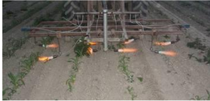
Figure 2.7. Intra-row flame directs flame to weed plant (Source: http://www.bhu.org.nz/ ).
