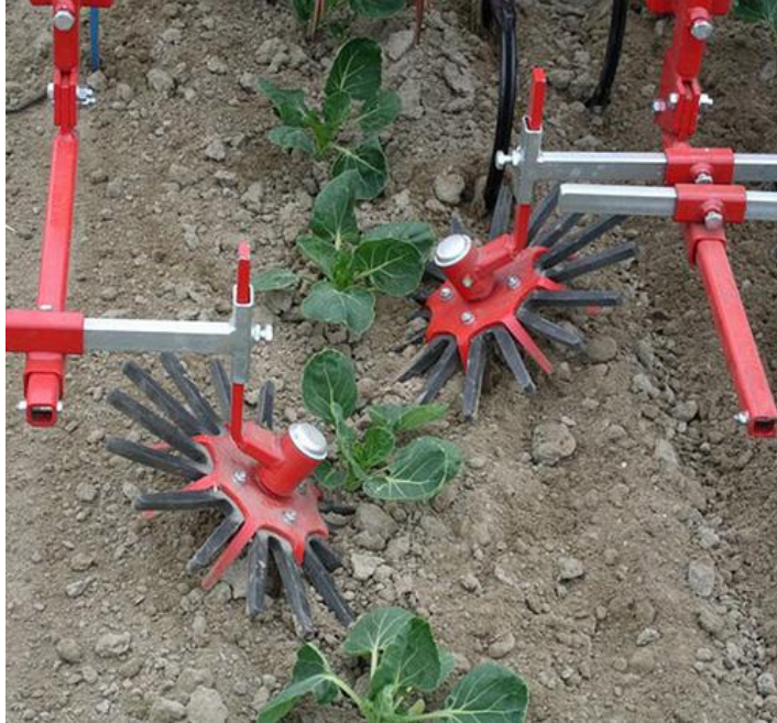
Figure 2.5. Finger weeder uses two circular shaped rotating disk with flexible rubber spikes to control weed plants (Source: http://www.suttonag.com ).
