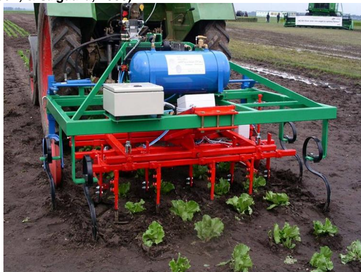
Figure 2.9. Sari Radis uses light sensor to detect crop and guides a hoe in and out of the crop row.
