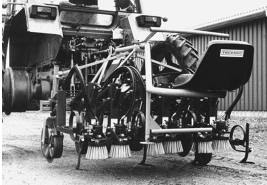
Figure 2.3. Brush weeder needs precise maneuvering by an operator to eliminate weed and avoid contact with crop plants (Melander, 1997).
