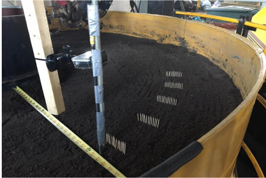
Figure 3.3. Five sets of each with 15 woods cylinders was set up in the soil bin for a trial.
