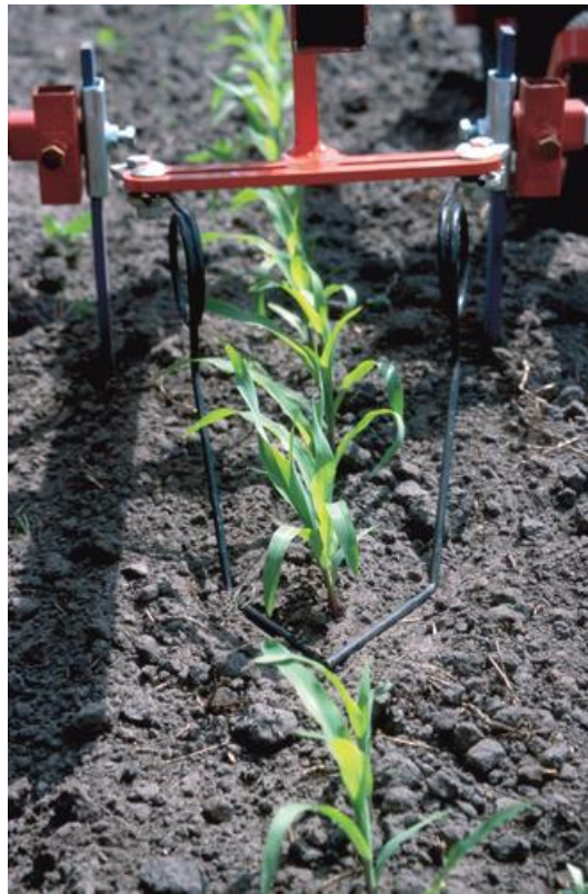
Figure 2.4. Torsion weeder uses bending steel spring tines to reach neighboring weed plants (Van der Weide et al., 2008).
