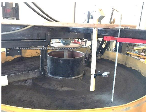
Figure 3.1. The circular soil bin with controlled speed used for the tine-soil interaction experiment located at AMSL at Iowa State University with a diameter of 2.44 m.
