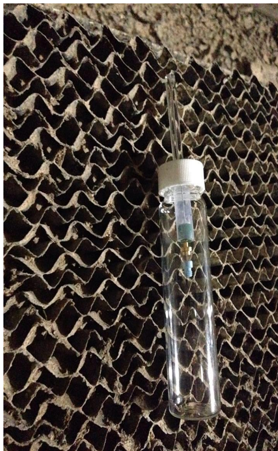
Figure 5A Placement of the SPME fibers and the sorbent tubes in Farm 2.
