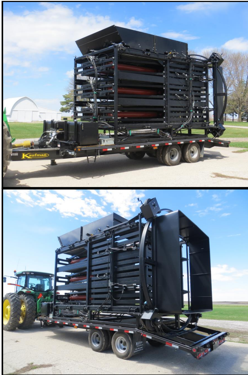
Figure 9.1: Large module builder prototype with all structural, hydraulic, and electrical components
