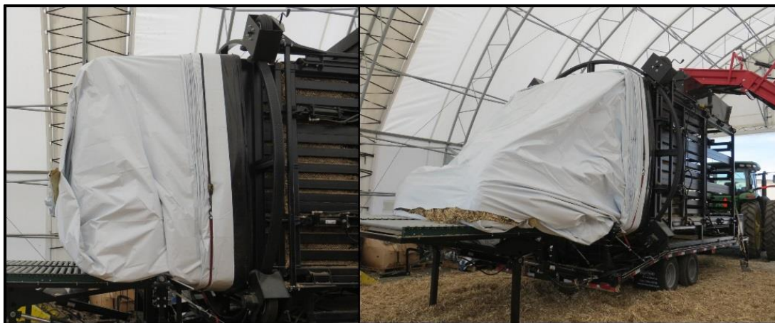
Figure 11.11: Module extrusion issue with falling flakes
