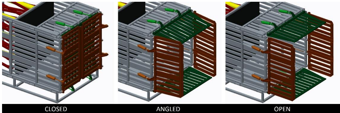
Figure 5.7: Three different operational door positions: fully closed, angled to specified compaction angles, or fully open
