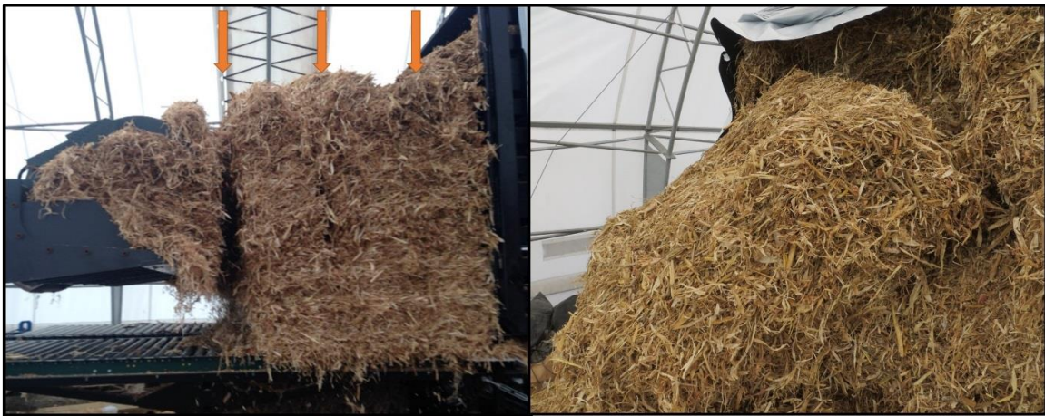
Figure 11.8: Flake formation within compacted large module
