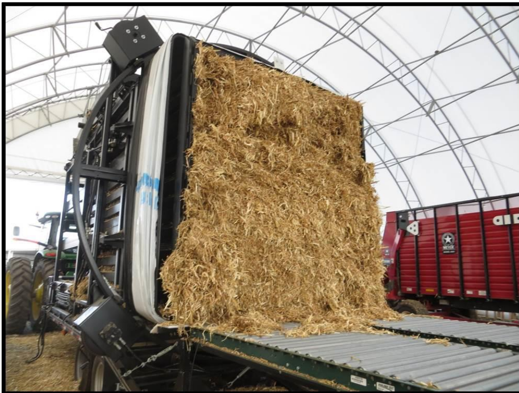
Figure 12.1: Large module builder machine with full module in chamber
