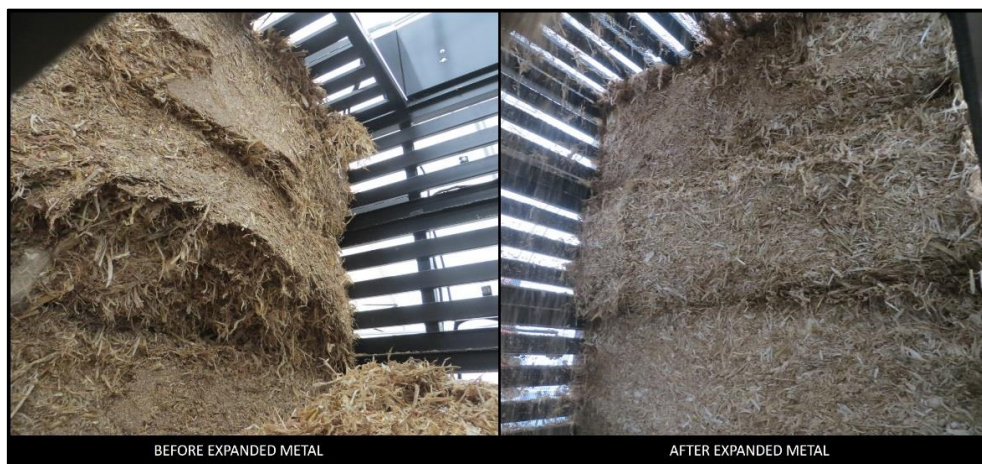
Figure 11.7: Difference in module face quality before and after addition of expanded metal inside compaction chamber
