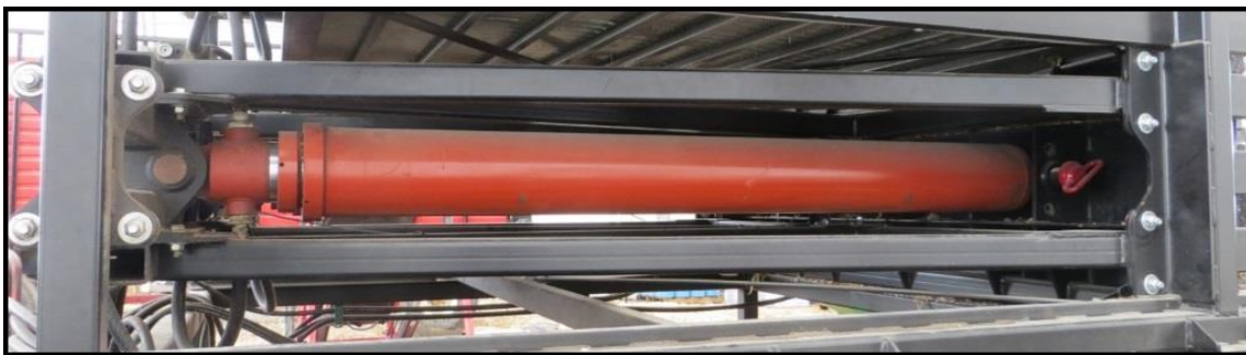
Figure 7.2: Double-acting telescopic hydraulic cylinder to actuate plunger
