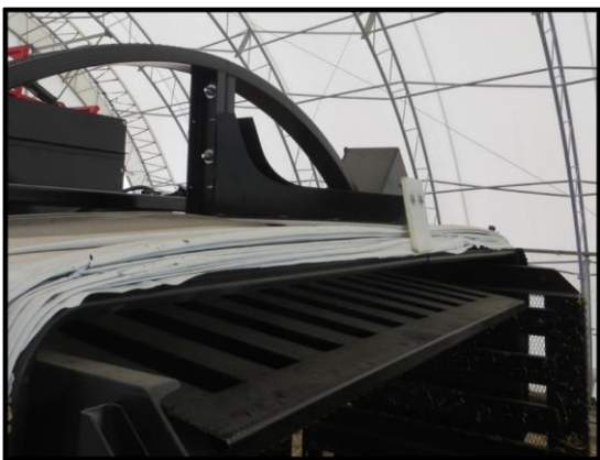
Figure 9.6: Silage bag retainer mounted to rotating hoop
