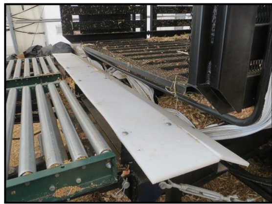
Figure 9.7: Ramp to bridge gap between door outlet and roller bed
