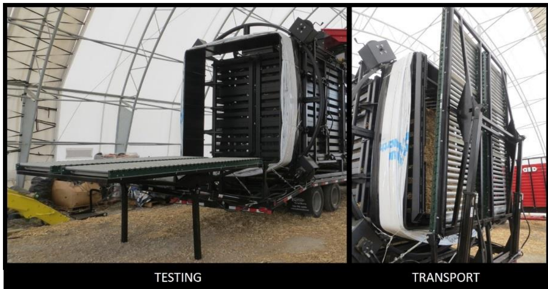
Figure 9.2: Finished module platform in both testing and transport positions
