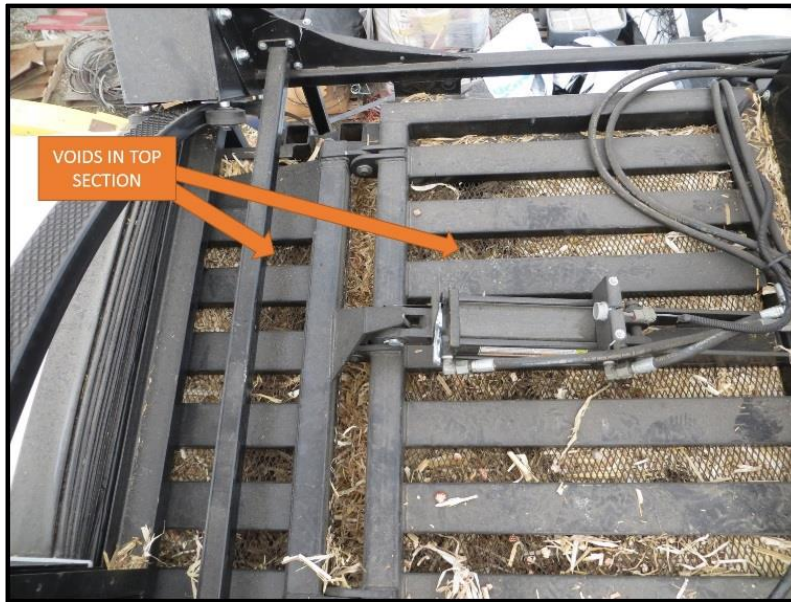
Figure 11.9: Effect of lagging top plunger from pinch point at end of throat opening
