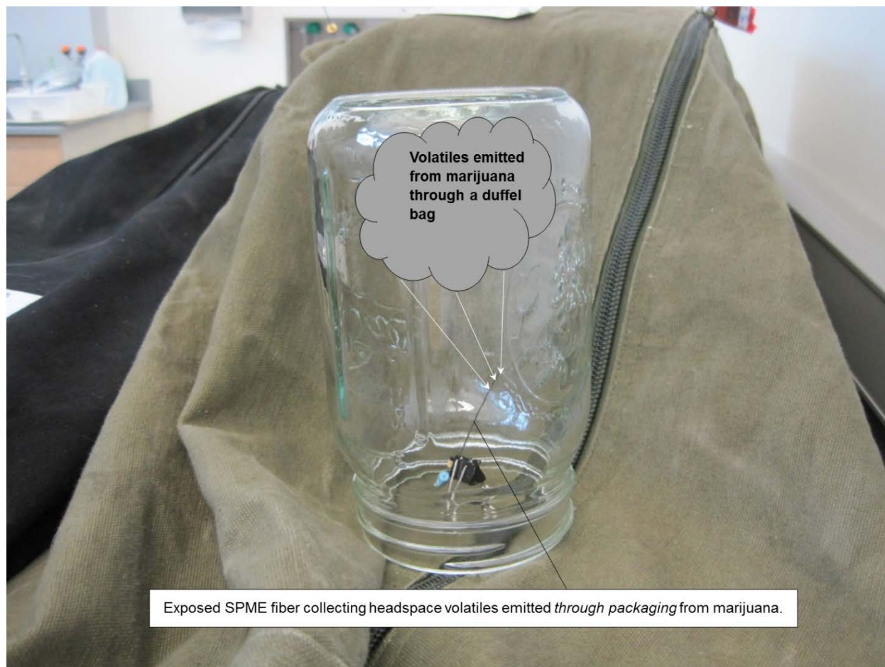
SI Figure 2. Static headspace sampling of VOC at room temperature from marijuana emitted through a duffel bag. A US military-style duffel bag containing ~50 kg of marijuana was seized and tagged as evidence. The SPME fiber was exposed and propped up by a metal binder clip, inside an over-turned, pre-cleaned 16 oz glass mason jar. This ad hoc apparatus created a headspace sampling chamber to collect VOC emitted from the marijuana and through the duffel bag over a period of 68 hours. The fiber was transported back to the lab for analysis as described in the caption of SI Figure 1.
