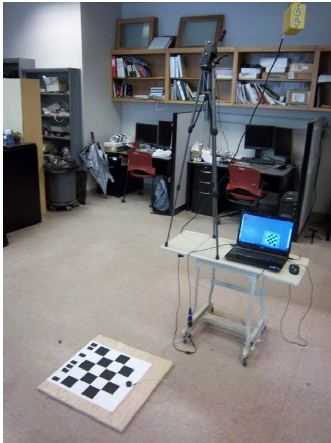
Figure 3.19. The setup of the angle measurement experiment with the Z axis of the target parallel to gravity
