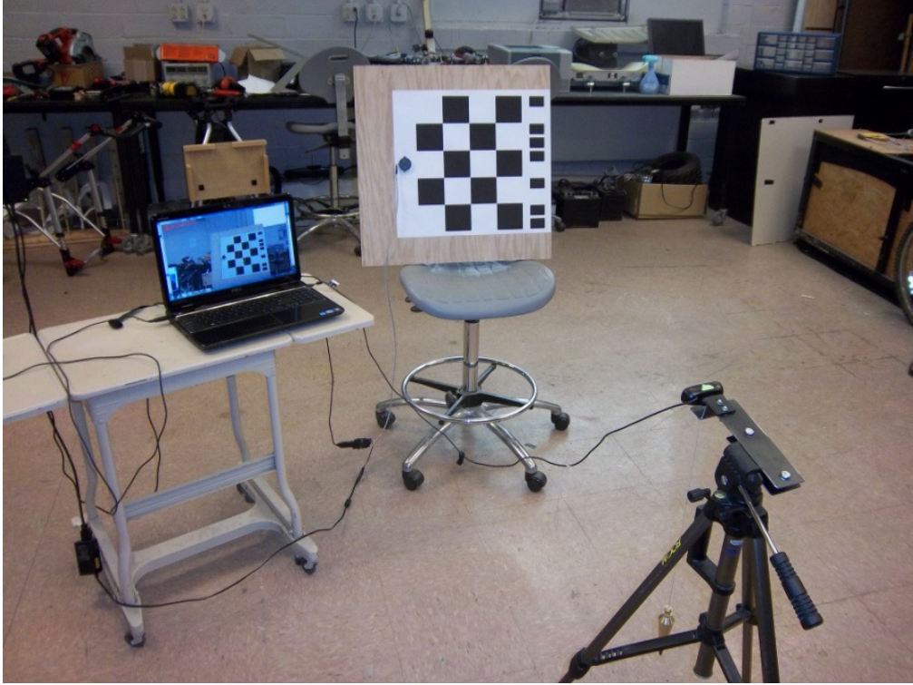
Figure 3.21. The setup of the angle measurement experiment with the X axis of the target parallel to gravity
