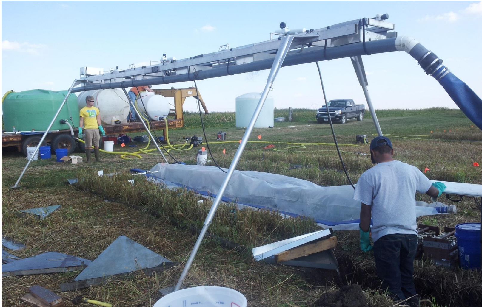
Figure 3.4: Photograph of a rainfall-runoff simulation in progress showing the experimental setup.
