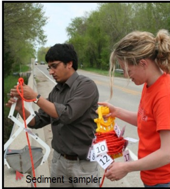
Figure A1. Sample collection devices: stream water samples were collected using horizontal polycarbonate water bottle (left), and streambed sediment samples were collected using Shallow Water Bottom Dredge Sampler (right).
