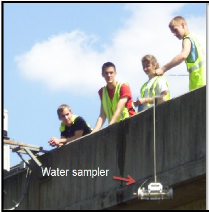
Figure A1. Sample collection devices: stream water samples were collected using horizontal polycarbonate water bottle (left), and streambed sediment samples were collected using Shallow Water Bottom Dredge Sampler (right).
