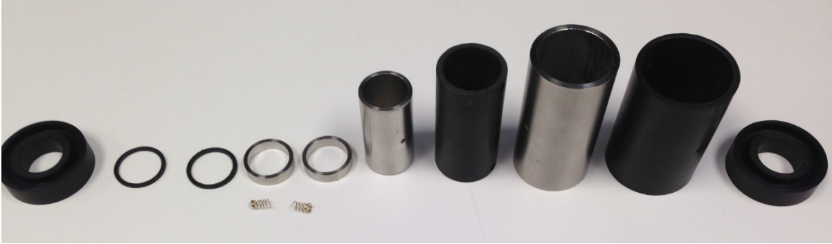
Figure 8. The sensing unit's outer electric electrode assembly consisted of 12 parts made from metal and polymer materials. The sensing unit also consisted of a rod and two rod holders (not shown).
