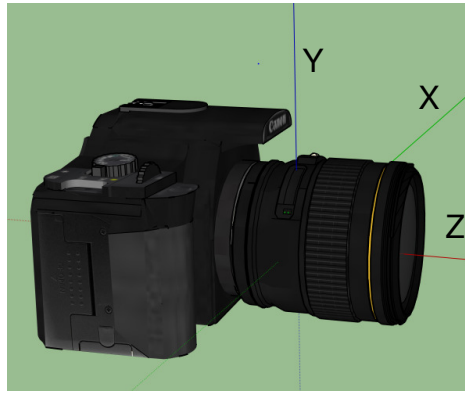
Figure 3.5. Canon camera coordinate
