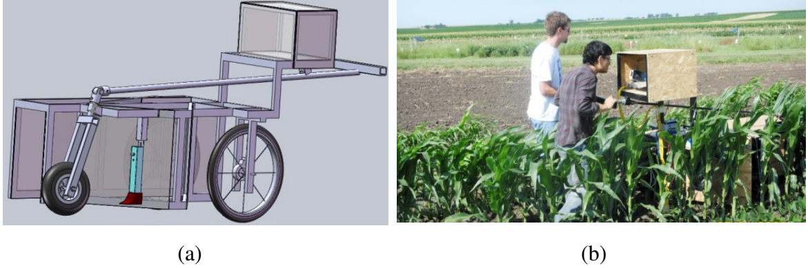
Figure 3. Three-wheeled inter-plant distance measurement platform: (a) CAD model showing an encoder attached to the rear wheel and a leveler mounted in front of it; and (b) the real cart in action in one of the test fields
