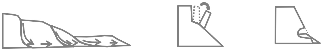
(a) Deep-seated Slump failures
