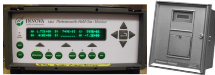
Figure 3.4. INNOVA 1412 photoacoustic multi-gas analyzer for CO 2 concentration and dew point measurements (left) and Rosemount 755A paramagnetic analyzer for O 2 concentration measurement (right).
