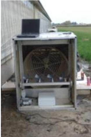
Figure 2.5. The in-situ ventilation fan calibration device used to determine air flow rate of the exhaust fans (left) and example performance curves for the same fan measured at intervals during the project.
