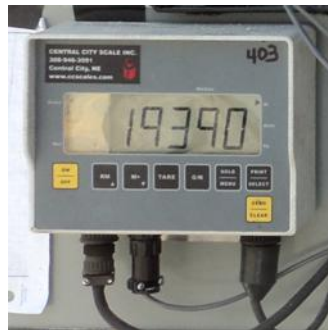
Figure 12: Scale head for weighing system mounted in grain cart enclosure
