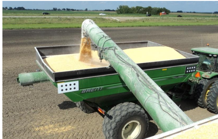
Figure 70: Brent 1088 grain cart used during dynamic field testing of the decision support system
