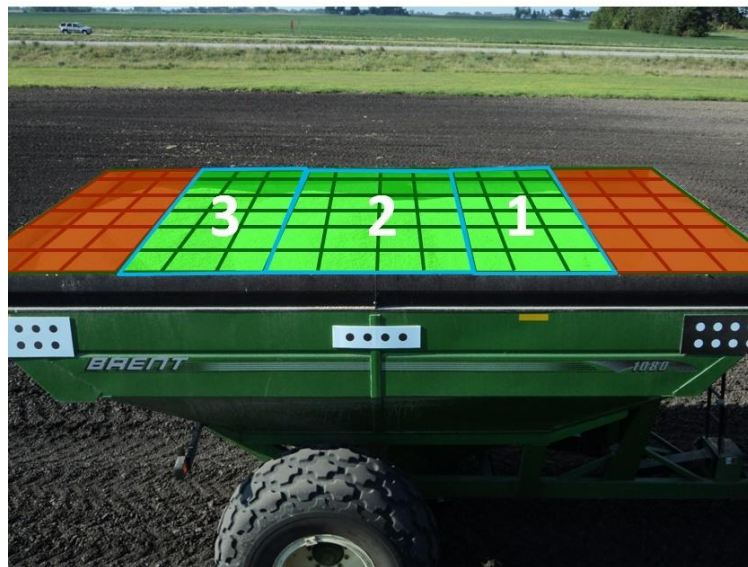
Figure 4: Grain cart overlaid with front and rear edge dead bands and three fill zones; grain can be delivered to the fill zones highlighted green, but the auger moving into a red zone causes it to disengage
