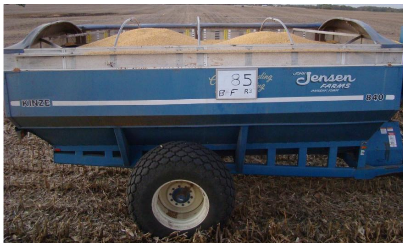
Figure 3: Kinze 840 bu grain cart used at Iowa State University as the standard size container to serve as the baseline for percentage-based fill height calculations
