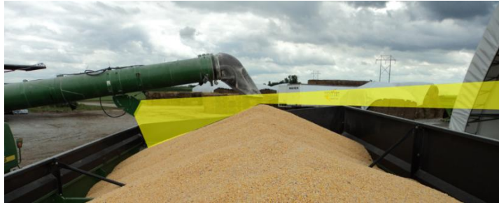
Figure 29: View from an auger-mounted stereovision camera of the grain height on the far half of the cart obstructed by a peak in the center ( Situation 4 )
