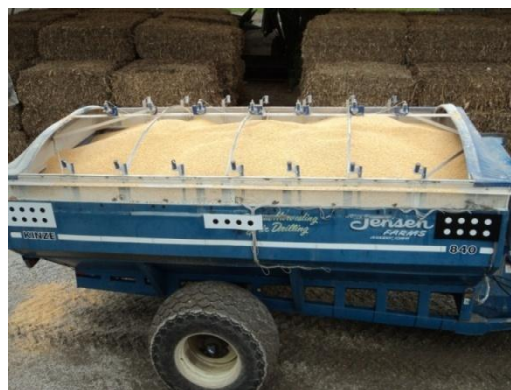
Figure 6: Kinze 840 bushel capacity grain cart with white side wall extensions increasing the capacity to about 1000 bushels
