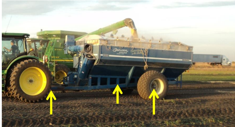
Figure 11: Kinze grain cart with arrows indicating the locations of load cells for the weighing system
