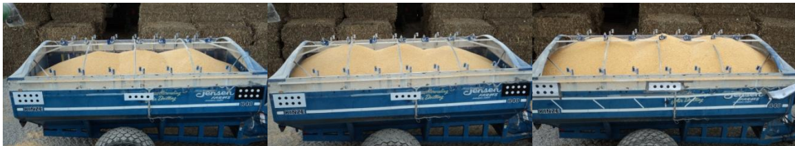
Figure 34: Grain carts filled with three fill zones to an average height of -40 cm (left), -25 cm (center), and -10 cm (right), as determined by the average height measured in Columns 3, 5, and 7 of the fill grid; Columns 3, 5, and 7 were at the center of the three fill zones
