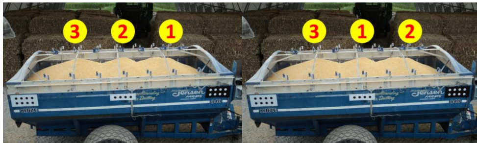
Figure 39: Numbered order in which grain was delivered to discrete fill zones of the grain cart; Front-Middle-Back (left) and Middle-Front-Back (right)
