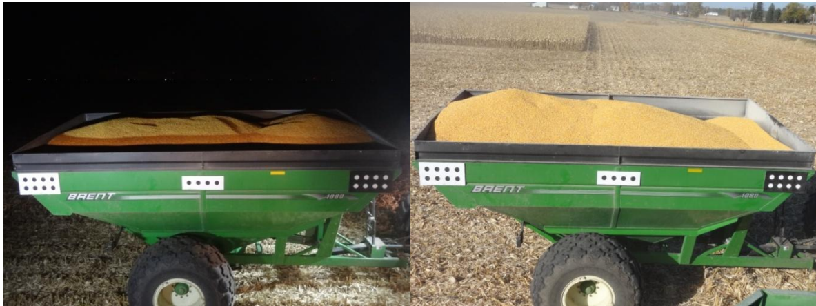
Figure 85: Brent grain cart filled with a 95% (left) and 100% (right) desired fill level in the decision support system
