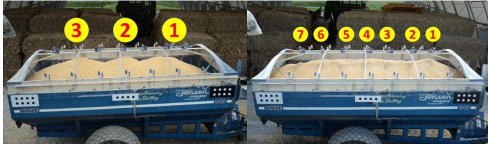
Figure 40: Grain cart filled using three fill zones (left) and seven fill zones (right) in a Front-Middle-Back zone filling order
