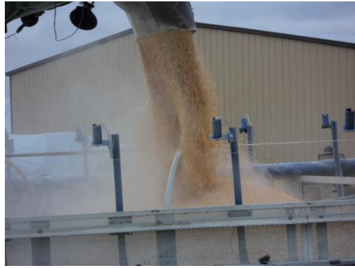
Figure 27: Grain being delivered directly onto an ultrasonic sensor causing an erroneous output for the distance measurement (Situation 1)
