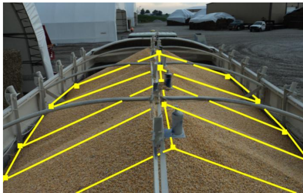
Figure 13: Using grain height measurements at three points to estimate the grain surface profile
