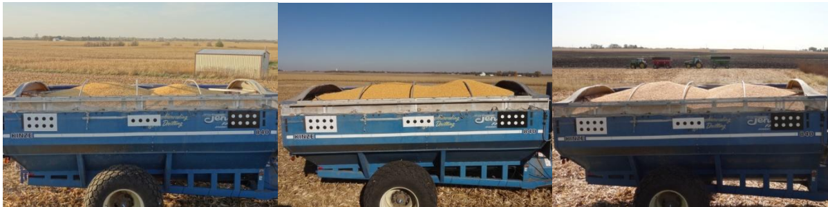
Figure 83: Kinze grain cart filled with a 95% (left), 100% (center), and 105% (right) desired fill level in the decision support system
