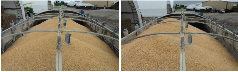
Figure 38: Grain cart filled with a lateral distance between the combine and grain cart of 590 cm (left), placing the peak directly below the middle row of sensors, and 520 cm (right), placing the center of the peak closer to the far edge
