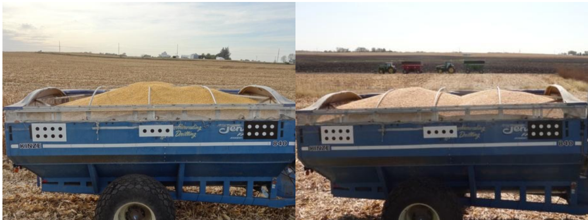
Figure 87: Kinze grain cart filled with the center point of the first and last fill zones offset one cell (25 cm) outward from the actual center of the zones; grain is piled toward the middle with empty space at the front and back
