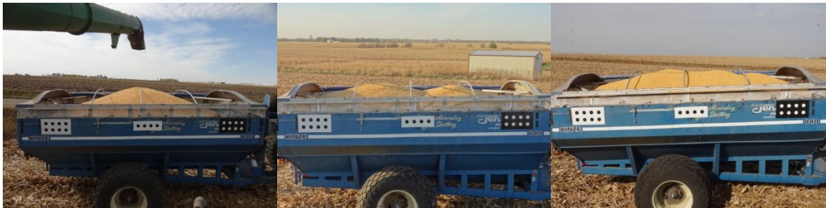
Figure 79: Kinze grain cart filled with one (left), two (center), and three (right) fill zones
