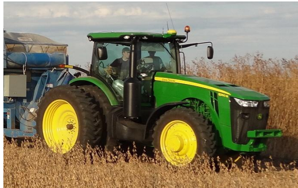
Figure 8: John Deere 8245R tractor used to tow the grain cart and power the onboard electronics
