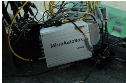
Figure 19: dSPACE, Inc. MicroAutoBox used for signal logging in ControlDesk and running the decision support system in the background without controlling auger actuations
