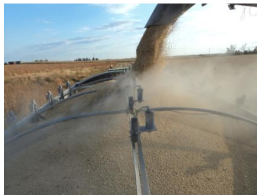
Figure 28: Grain being delivered to a grain cart with heavy dust conditions blocking the view of the grain pile by a stereovision camera mounted on the auger of the combine (Situation 3)
